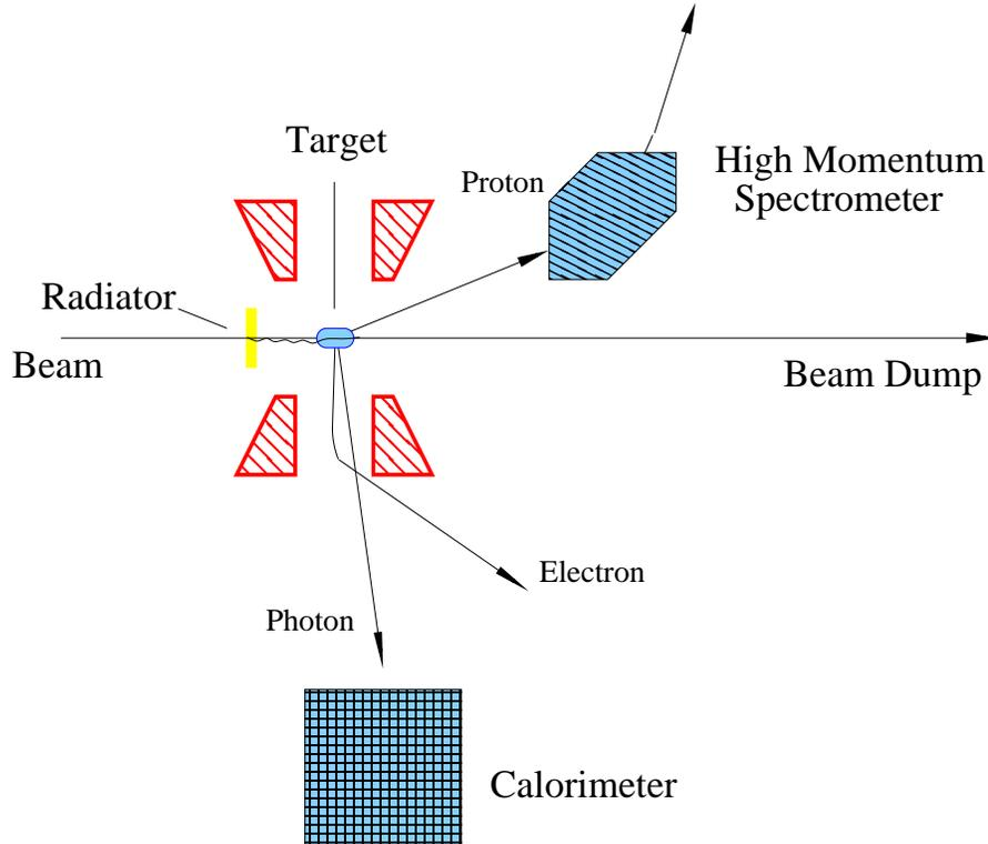
Figure 8: Schematic of the experimental setup. The target is longitudinally polarized (along the beam). The scattered photon is detected by NPS and the recoil proton is detected by the HMS. The scattered electron in the mixed photon-electron beam is deflected by the polarized target magnet.
