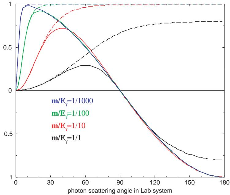
Figure 7: Klein-Nishina polarization observables  $A_{LL}$  and  $K_{LL}$ , shown by solid lines and dashed lines respectively, for different ratios of the electron mass to the photon energy as a function of the scattering angle in the lab system.
