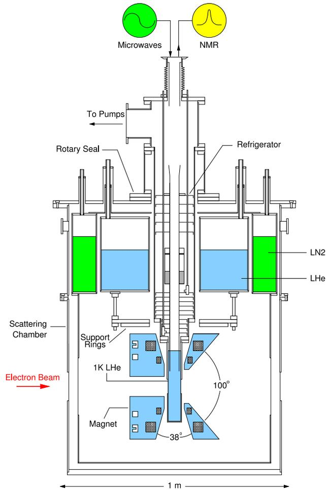
Figure 9: Cross section view of the polarized target.
