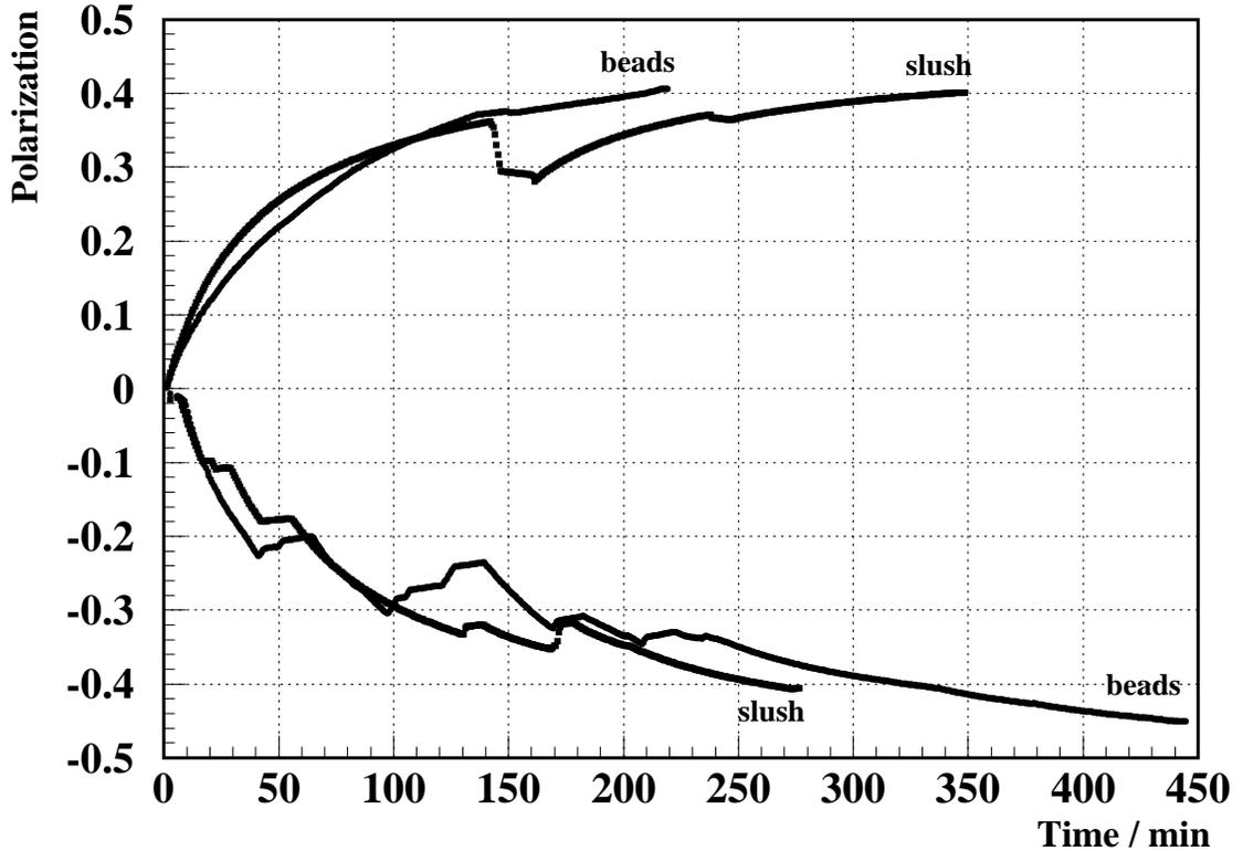
Figure 3:  $\text{ND}_3$  polarization with material recovered after the Hall C accident. The kinks are either due to loss of liquid helium or changes in the microwave frequency.
