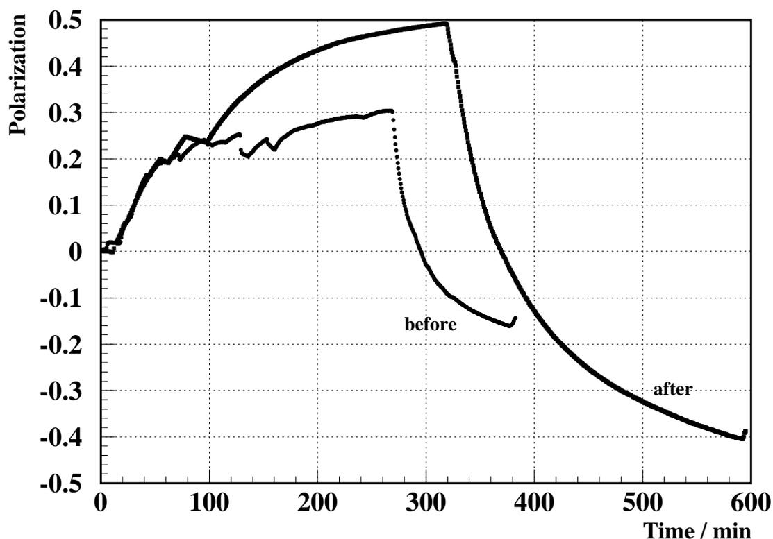
Figure 4:  $\text{ND}_3$  polarization, before and after tempering.
