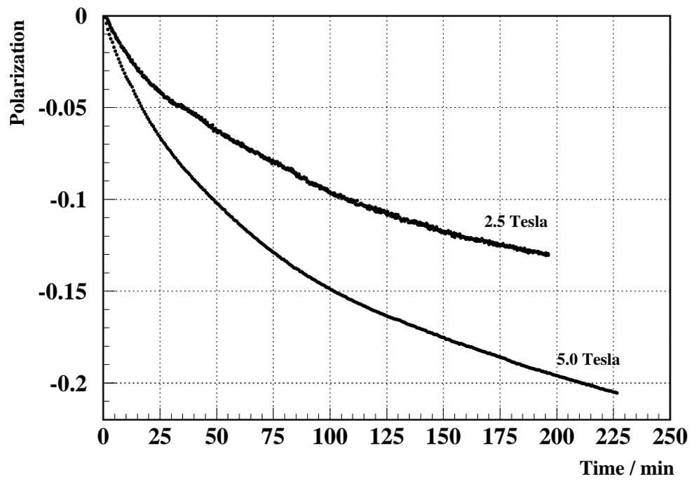
Figure 5: LiD polarization at 2.5 T, 5.0 T, and 7.55 T.
