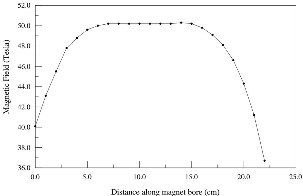
Figure 1: Hall probe measurement of magnetic field uniformity along central bore axis.
