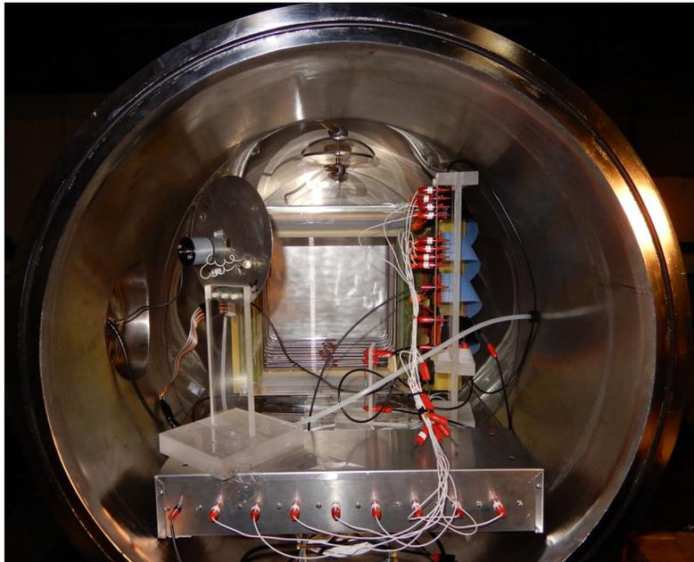
Figure 8 - The BDX-DRIFT-0.3m NITPC inside the vacuum vessel below the HHV feedthrough at the back. The Fe-55 source is seen on the left at the front. The cathode readouts are shown on the bottom and right.
