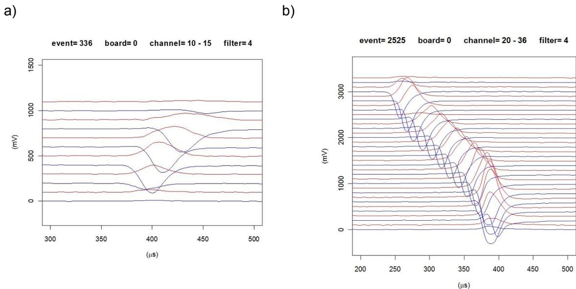
Figure 31 – a) A neutron event on DRIFT-IIe with interspersed anode and field wires. Blue is anode, red is field wire. Some digital filtering was used to remove noise. b) An alpha event in DRIFT-IIe. All events taken with a non-minority carrier gas.
