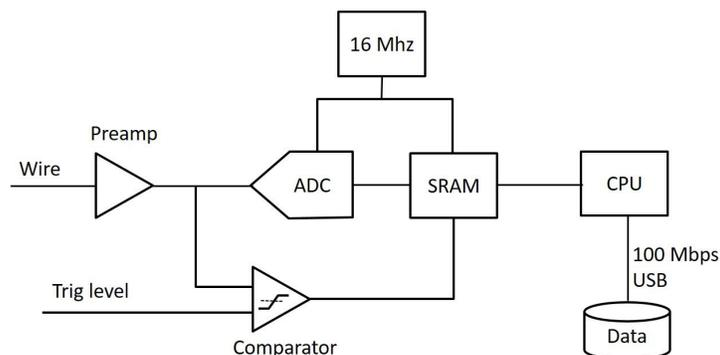
Figure 29 - Block diagram for DAQ v2.
