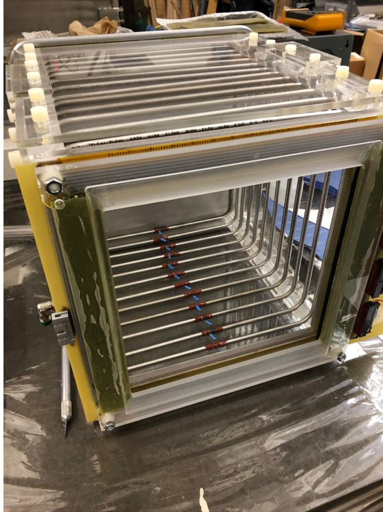
Figure 7 - The BDX-DRIFT-0.3m NITPC on the lab bench. The MWPC is towards the front. The  $\frac{1}{4}$ " field cage rings and connecting resistors are seen through the MWPC wires (not visible in photo). At the back is the Al cathode.
