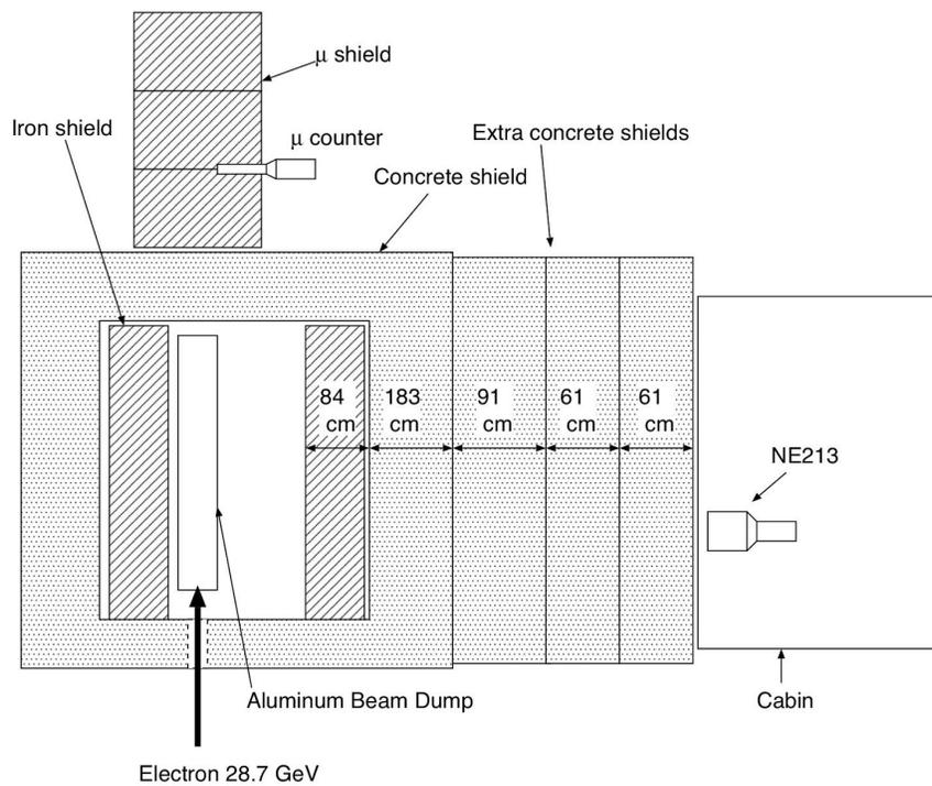
Figure 20 - The experimental setup for measurement of neutrons emanating from a beam dump at SLAC [38].
