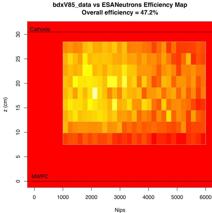
Figure 14 - The efficiency map for the ESA run. Each box shows the efficiency for detection at that location in the fiducial volume.
