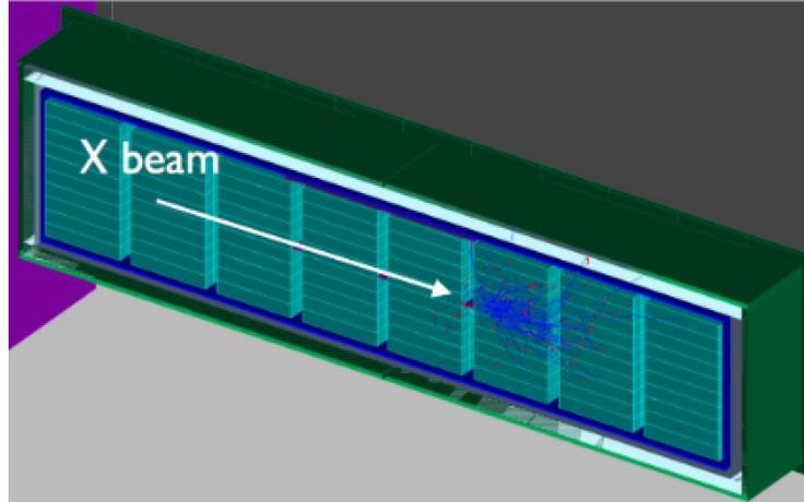
Figure 2 - The BDX detector as implemented in GEANT4. The OV is shown in green, the IV in gray and the lead vault in blue. Crystals arranged in 8 blocks of 10x10 are shown in light blue. A simulated electromagnetic shower from a  $\chi$ -electron scattering in the Ecal is also shown.
