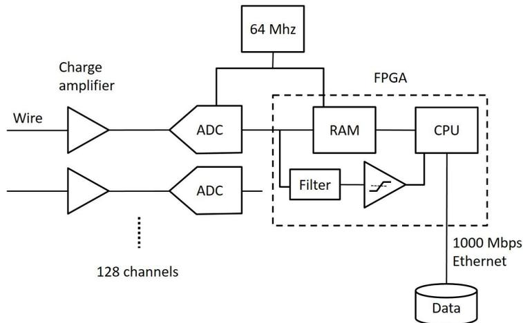
Figure 32 - Block diagram for DAQ v3
