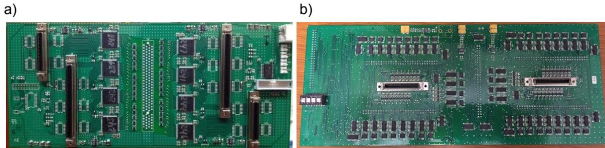
Figure 30 - a) Oxy/BNL 120 channel front-end board. b) Oxy 40 channel digital acquisition board.
