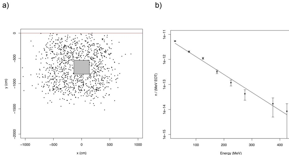
Figure 22 - a) Plot of xz coordinates of 1,072 neutrons passing a dirt plane 235 cm from the beam dump. The square in the middle is the iron shielding. The brown horizontal line shows ground level. b) Spectrum of neutron energies at the dirt plane.
