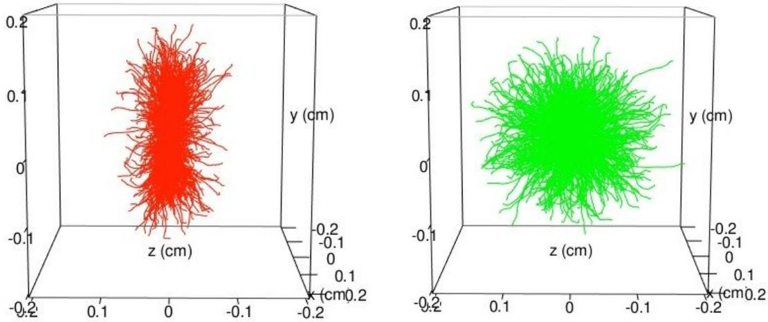
Figure 25 - a) Tracks produced by 1,000 50 keV S recoils originally oriented perpendicular to the beam or z axis according to an SRIM [23] simulation. b) Tracks produced by 1,000 50 keV S recoils oriented randomly as a comparison background. For scale the surrounding boxes are 4 mm in all dimensions.
