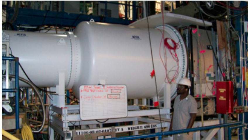
Figure 11: A photograph of the \sim 5 m long, two stage vacuum chamber used during the PRad experiment (left). A photograph of the 1.7 m diameter thin window at one end of the vacuum chamber (right).
