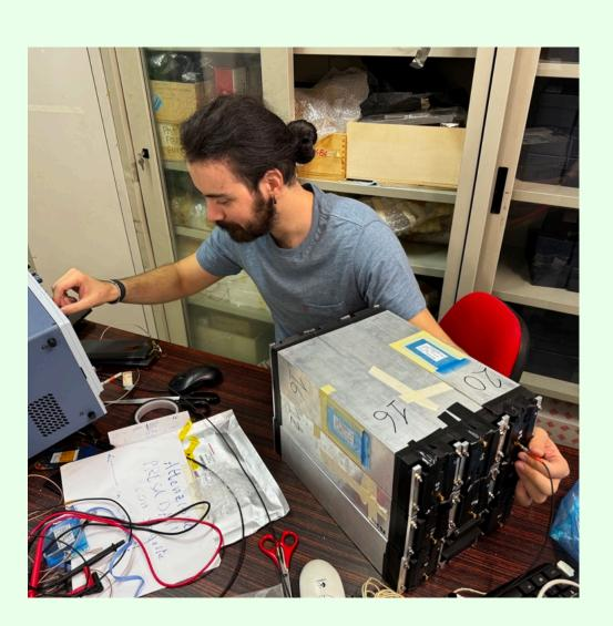
EM calorimeter: CsI(Tl) crystals read using SiPM Performed crystal characterization:
