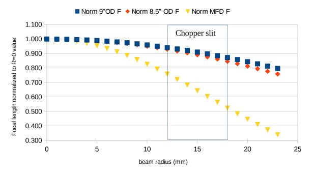
Chopper solenoid (MFD) and proposed replacements focal length variation vs beam location.
