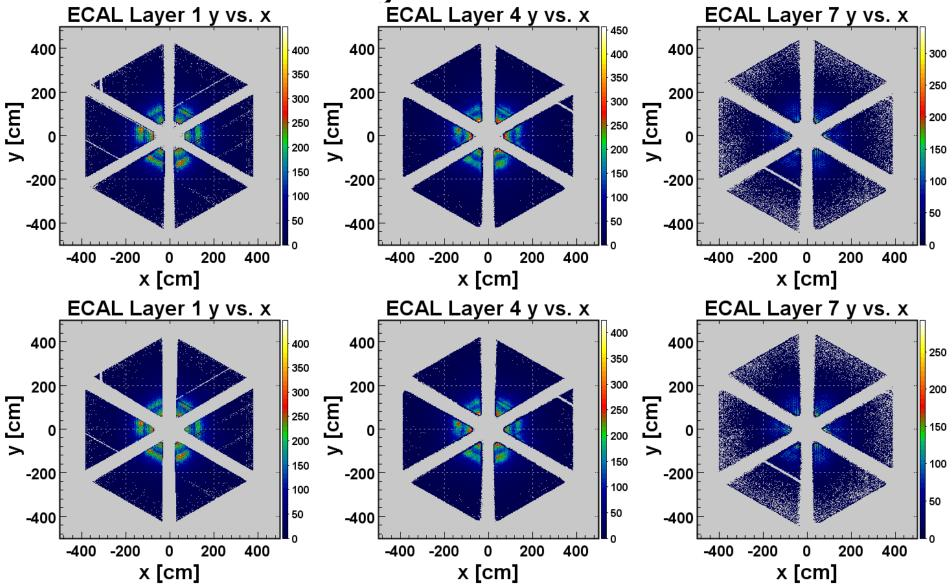
ECAL surface hit map of  $\gamma$  before (top) and after (bottom) implementing boundary fiducial cuts based on sampling fraction (SF).
