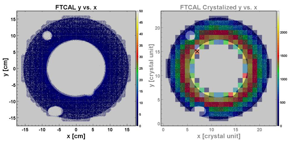
Elliptical boundaries are used to define the fiducial cuts (as shown as transluscent 2D hit maps) and are selected to smoothen the rough edges of the detector and the holes.
