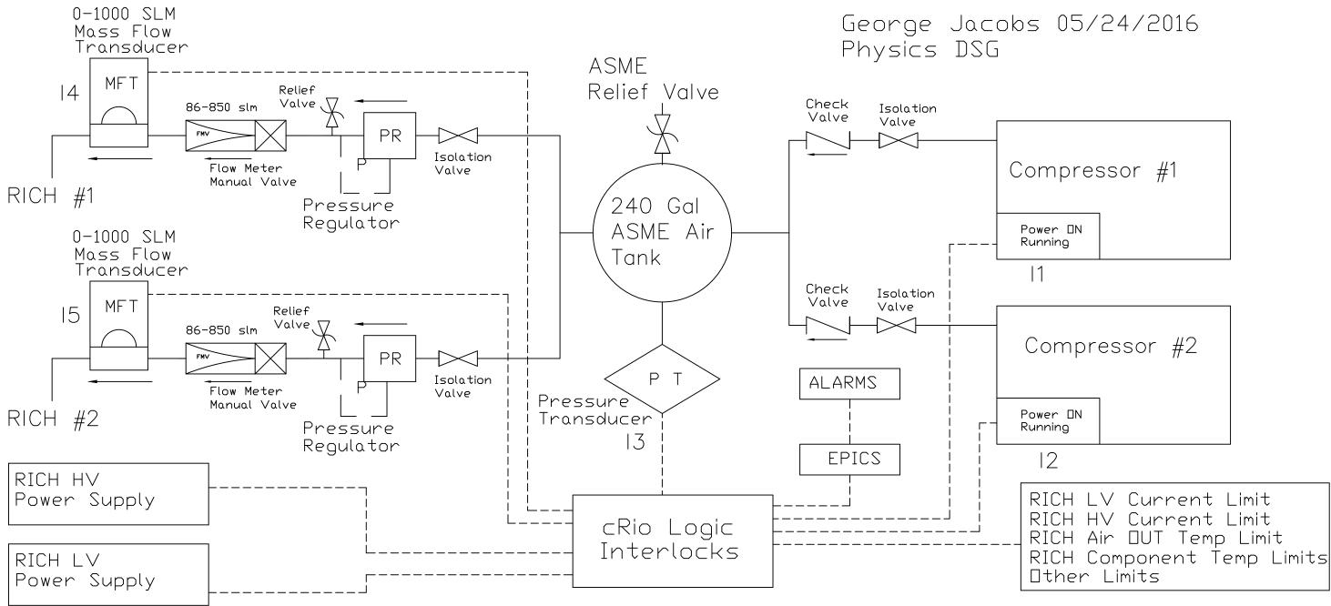
Cooling Circuit Interlocks for RICH HV and LV Power to be Enabled Air Compressor Power ON Interlock — I1 and/or I2 or PS Power is Disabled Air Pressure Interlock — I3 > 100 psi (TBD) or Power Disabled Air Flow Interlock RICH #1 Power — I4 > 250 slm (TBD) or Power to RICH #1 Disabled Air Flow Interlock RICH #2 Power — I5 > 250 slm (TBD) or Power to RICH #2 Disabled
