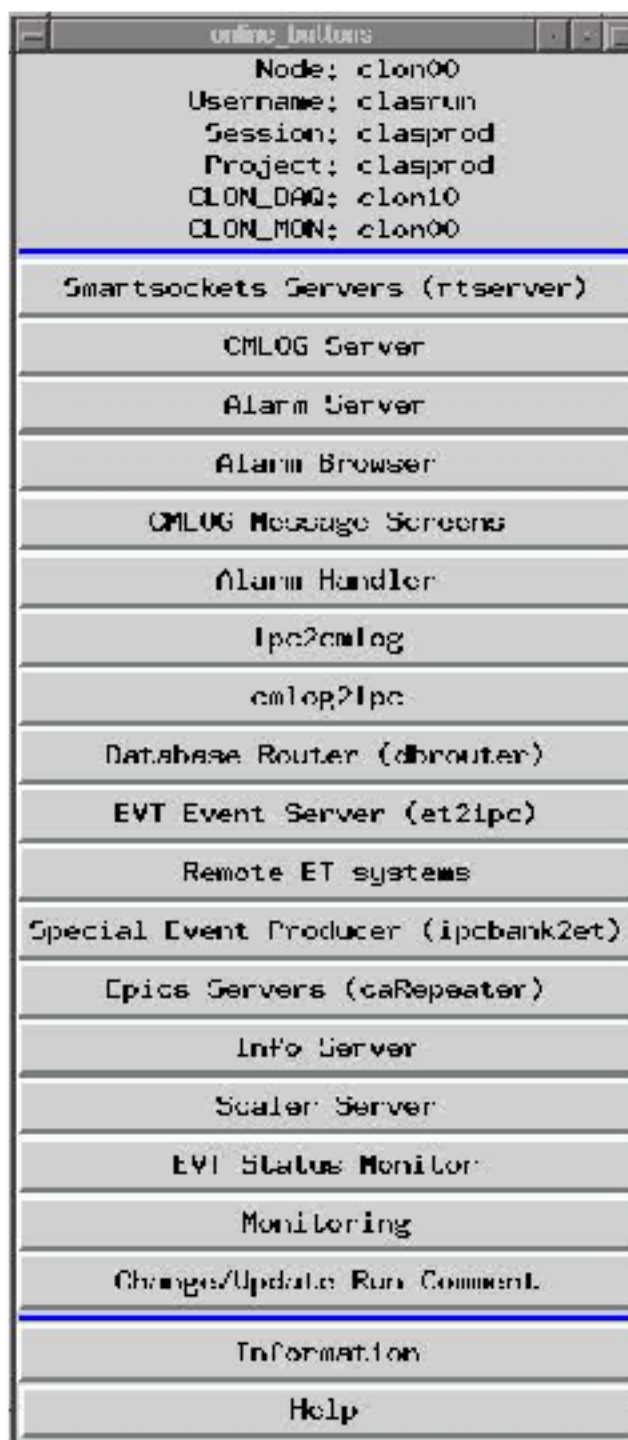
Figure 1: Screen capture of the graphical user interface (gui) for the online buttons. Bring this gui up by entering 'onlb' at the command line in the clasrun account.
