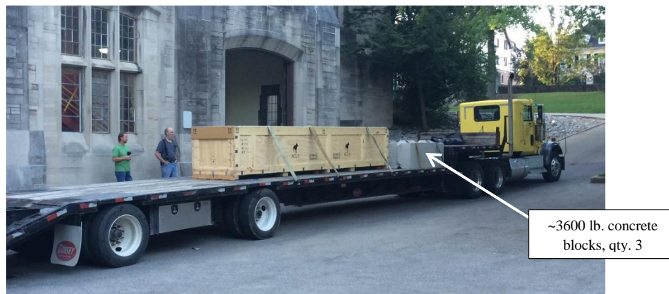
Figure 41 showing trucking equipment and set-up of second road test
