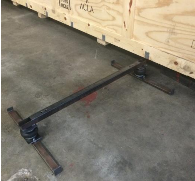
Figure 38 showing one of three outer crate suspension members
