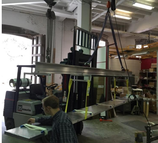
Figure 17 – Showing resonance test set-up for mock bar box
