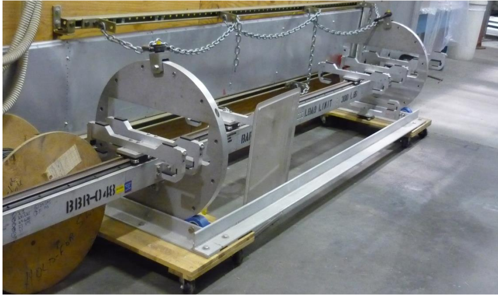
Figure 12 Specialized lifting and positioning fixture for bar boxes
