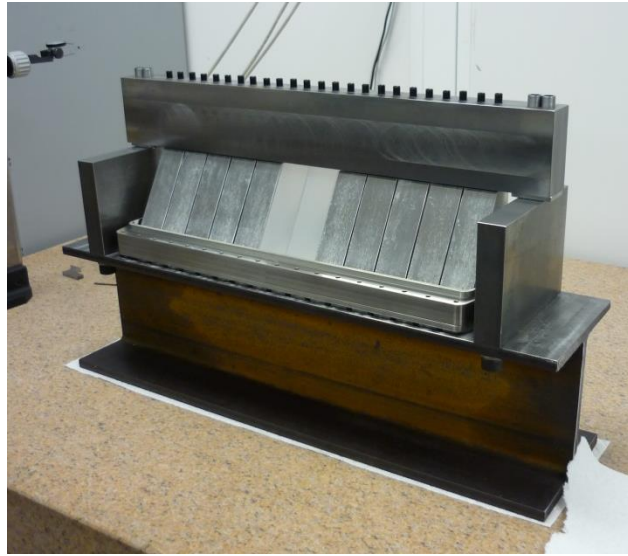
Figure 4 – Window Pressure Test Set-Up at full load
