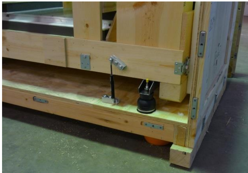
Figure 26 - showing air spring and damper – outer crate side removed for view
