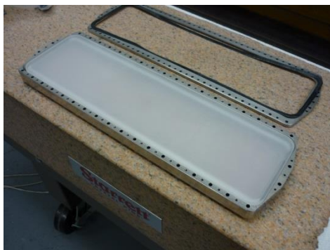
Figure 6 – Window, flanges and gasket following pressure test
