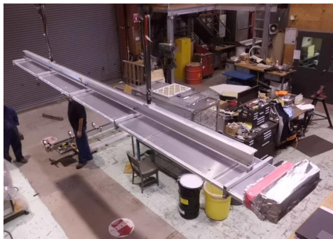
Figure 13 – Rigid lifting beam and bar box – SLAC
