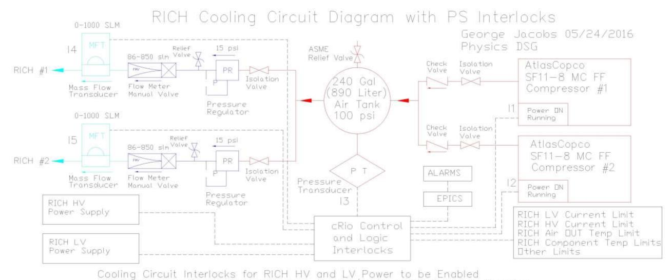
Air Compressor Power ON Interlock — I1 and/or I2 or PS Power is Disabled
