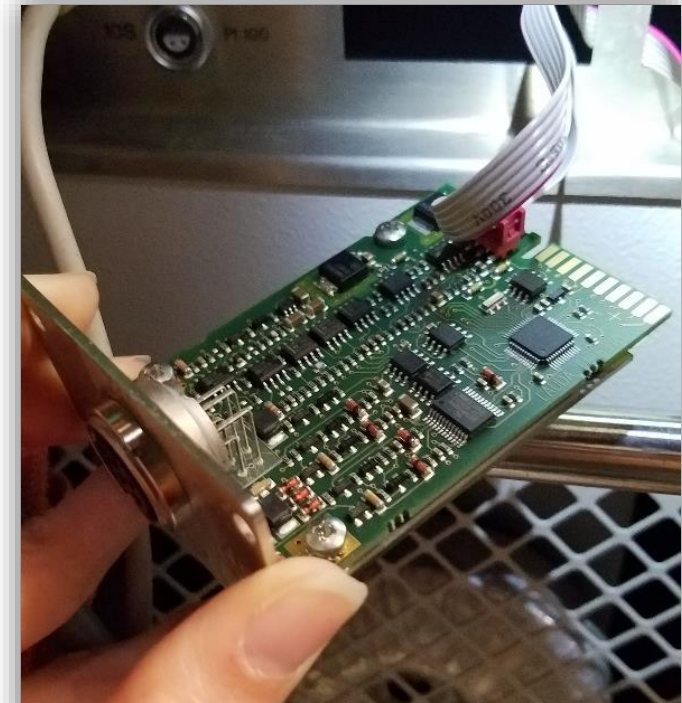
Analog card used for connection between hardware interlocks and chiller
