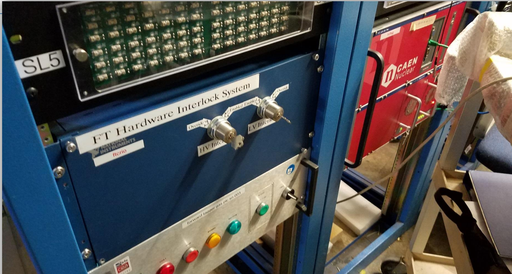
Hardware Interlock System installed in rack beside CAEN HV crate
