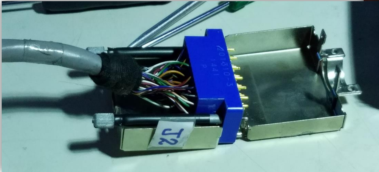
Pin modifications to HV cables
