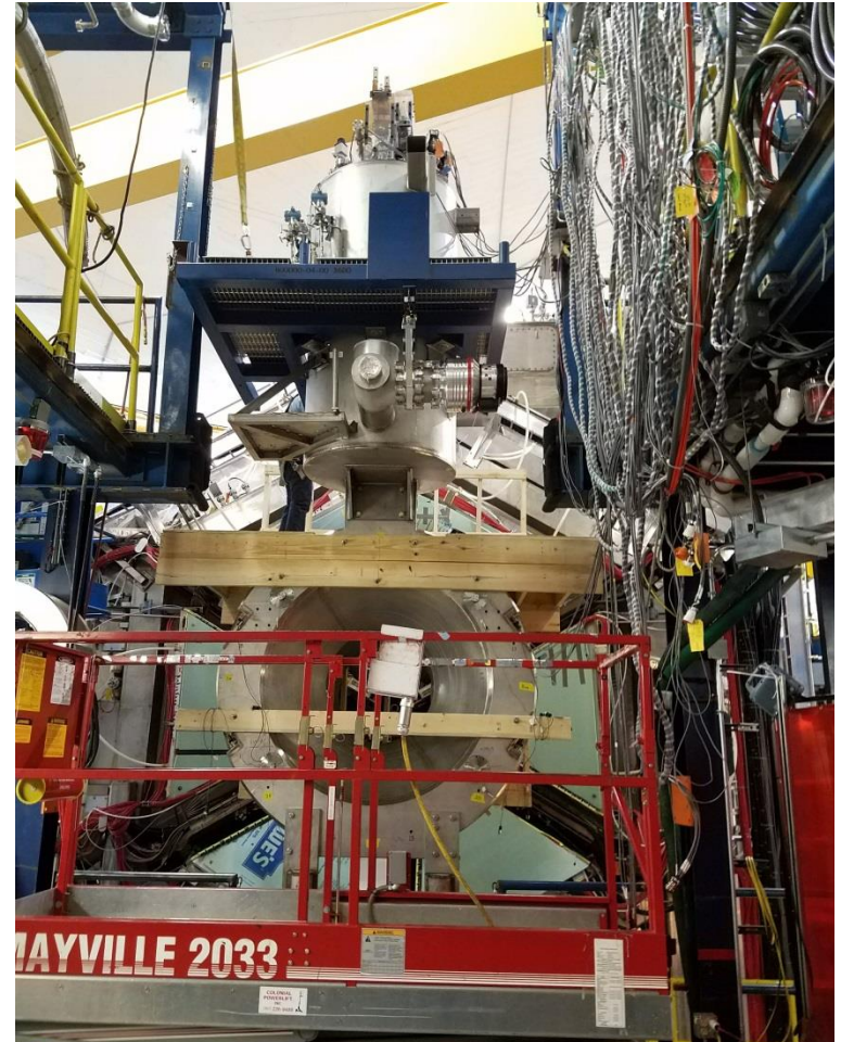
Solenoid final assembled with SST and Vacuum system
