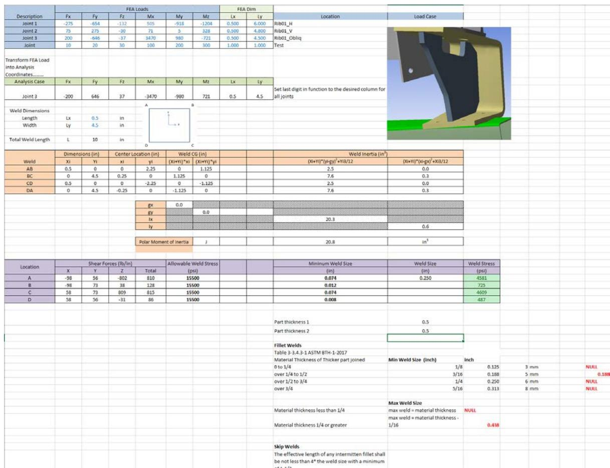
Figure 35: Weld Stress of the connecting flange
