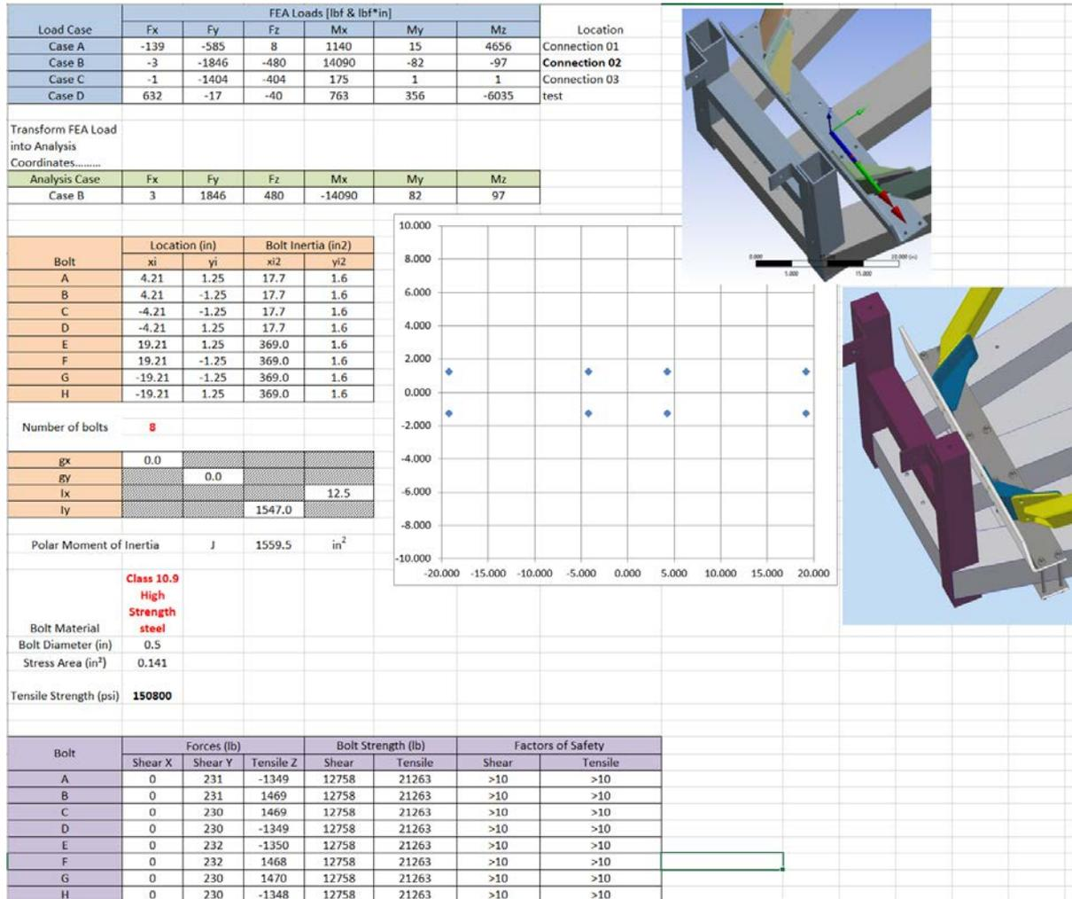
Figure 37: Bolted Stress at connection 02
