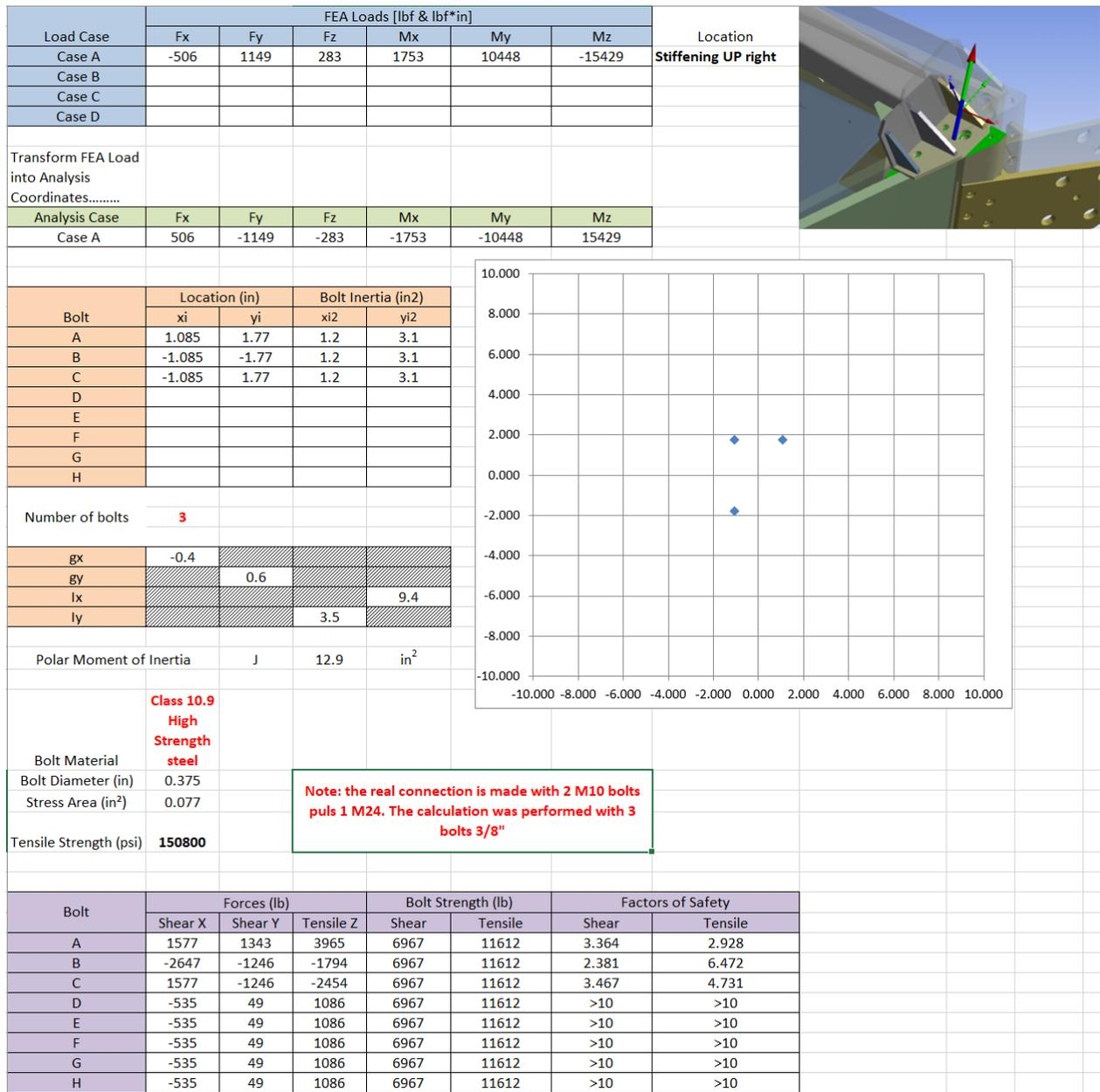
Figure 22: Bolted Stress at connection Stiffening Up Right
