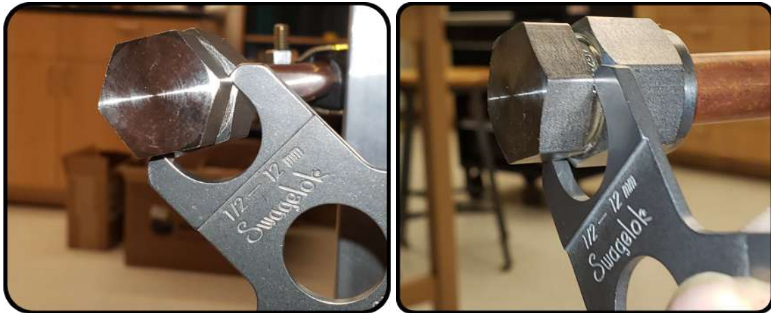
Figure 5: Picture example of the use of the gauge with the compression component.
