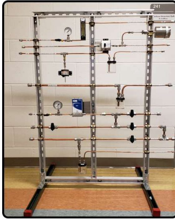
Figure 6: Completed RTPC and DMS gas panel photo.
