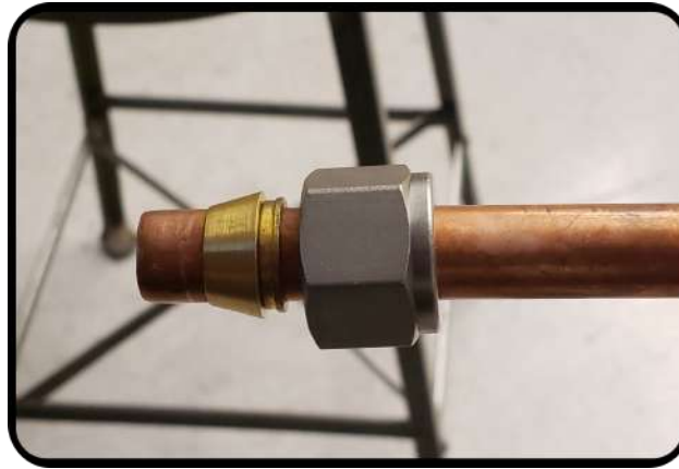
Figure 4: Picture of the brass ferrules used with the copper tubing in the gas panel with a stainless steel compression nut.
