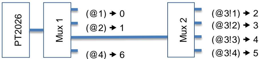
The same channel map is used for the Holding and Input Registers. The PT2026 MODBUS module supports up to 511 channels.
