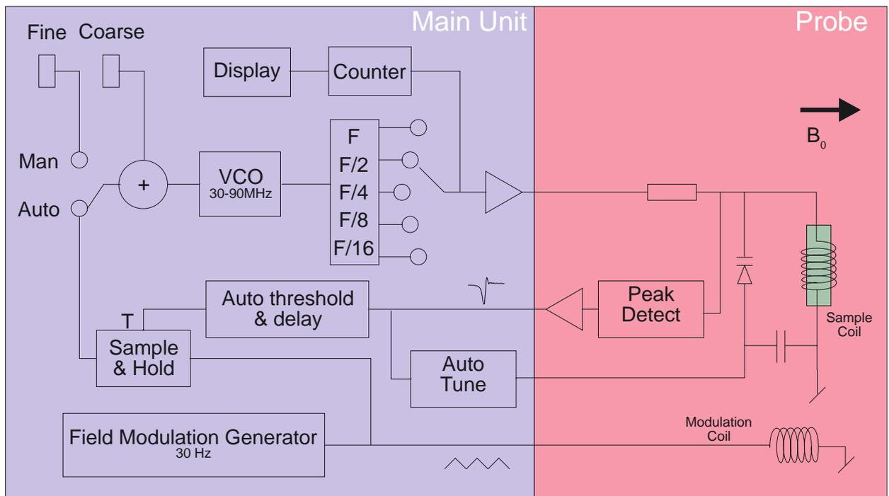
Figure 4. PT2025 functional block diagram.
