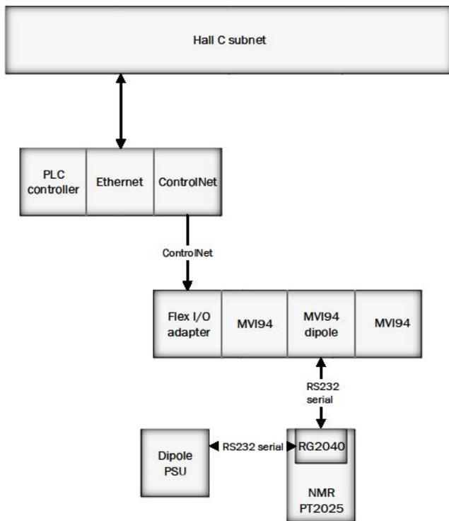
Current Hall C Dipole NMR Configuration for SHMS and HMS
