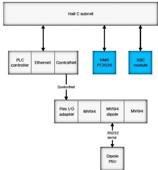
Proposed Hall C Dipole NMR Configuration for SHMS and HMS
