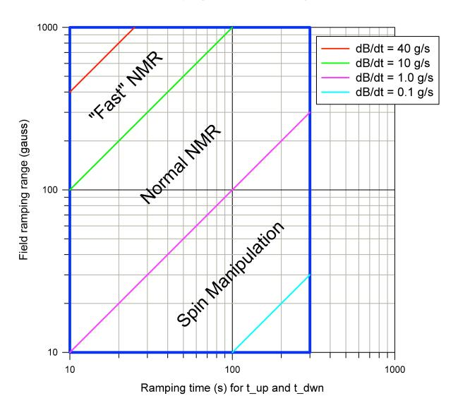
The parameter space for ramping HDice NMR magnets is shown as the blue rectangle. The field ramping range varies from 10 gauss to 1,000 gauss, while ramping time varies from 10 seconds to 300 seconds. Three "region of interest" are separated by 4 colored lines, representing 4 different ramping rates (40, 10, 1 and 0.1 gauss per second). Rates faster than 40 g/s and/or slower than 0.1 g/s are no interested. The center field for the ramping is set independently.
