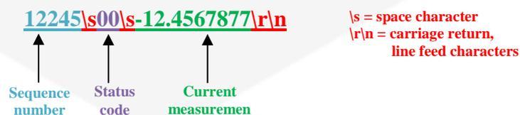
**Figure 14:** Data representation in Data-Logger mode
