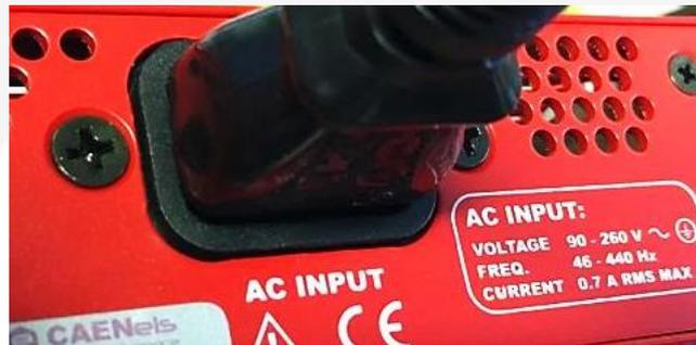
**Figure 4:** AC power cord connection
