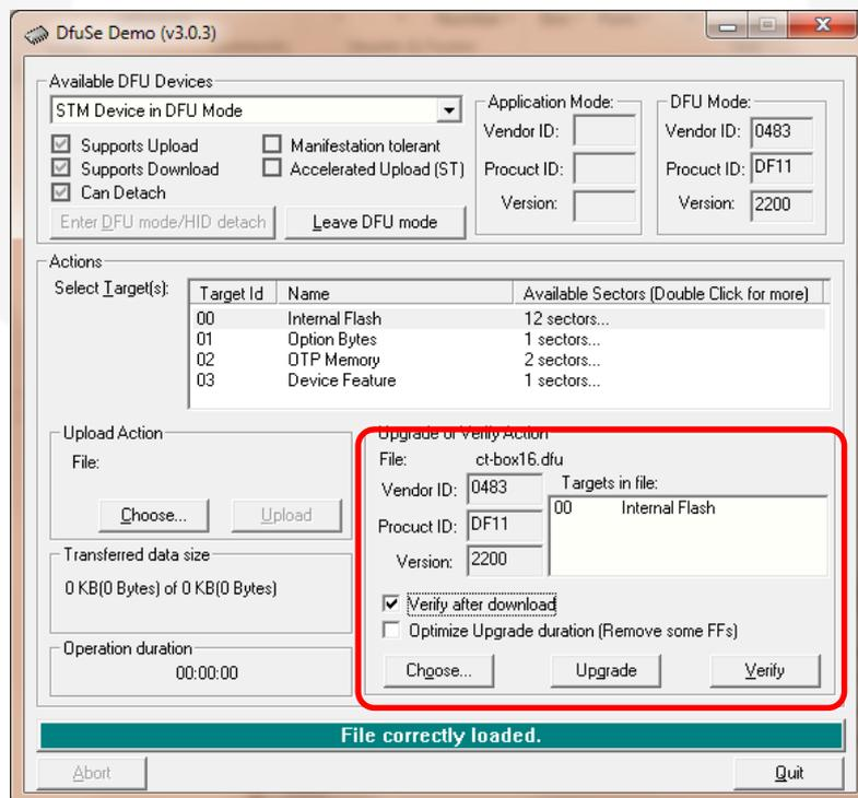
Figure 19: DfuSe Upgrade setup
