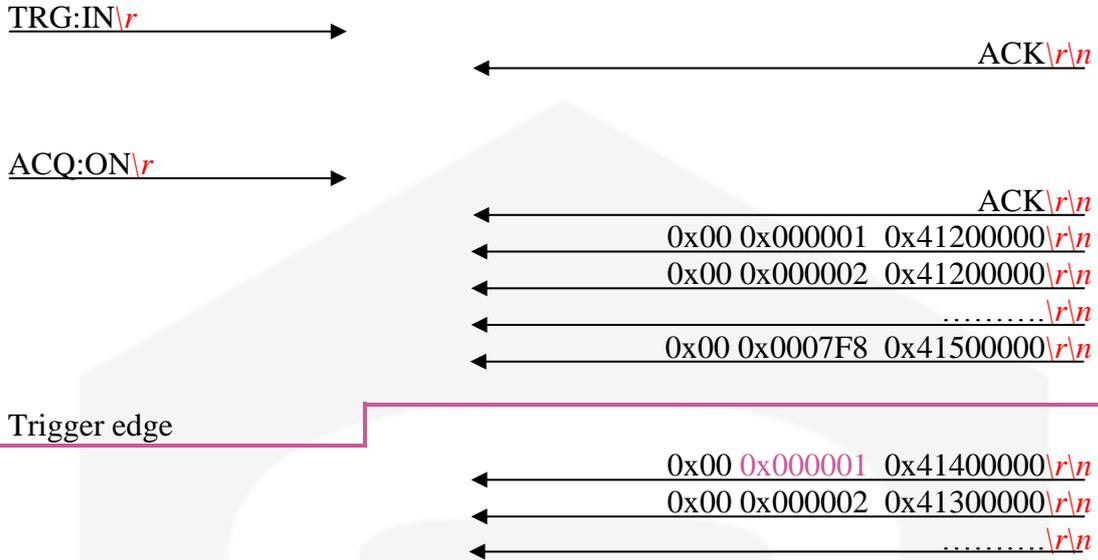
The command used to exit from the triggered acquisition mode is “TRG:OFF\r”. The command used to read the actual trigger setting is: “TRG:?\r”. The reply to the read command is in the following form: “trg\_setting\r\n”, where *trg\_setting* is “IN”, “OFF” according the actual trigger setting.
