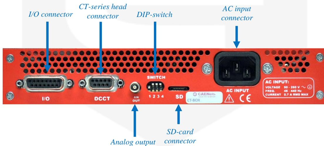
**Figure 2:** rear view of a CT-BOX unit
