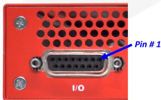
Figure 21: I/O connector
