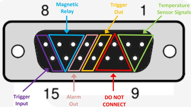
Figure 22: I/O connector description – rear panel
