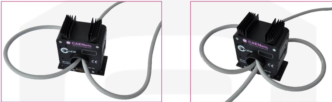
The PTURNS command allows to configure the number of turns applied to the CT-sensor head in order to scale the CT-BOX readings by the factor of turns  $N$ . The factory defined number of turns is #1 (no turns applied to the primary conductor).
