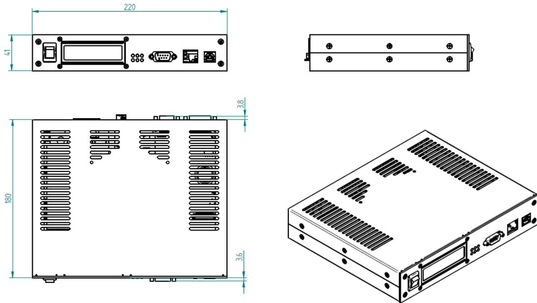
Figure 26: CT-BOX mechanical dimensions
