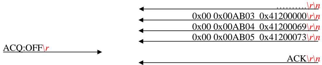
*ACQ ON example in Oscilloscope mode with PRINT enabled afterwards (note in this case the first acquisition 0x01 – 0x10 are not displayed, because the PRINT command is enabled afterwards):*
