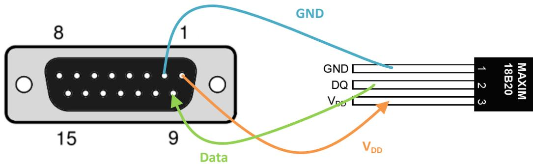
**Figure 23:** external temperature sensor connection to CT-BOX I/O connector
