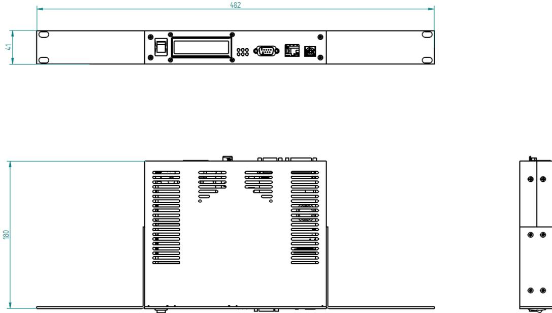
**Figure 27:** CT-BOX with Mounting Brackets
