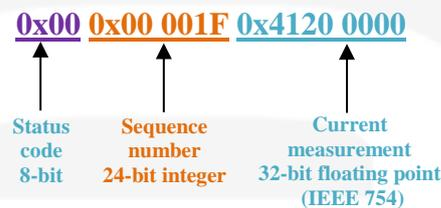
**Figure 12:** Data representation in the oscilloscope mode
