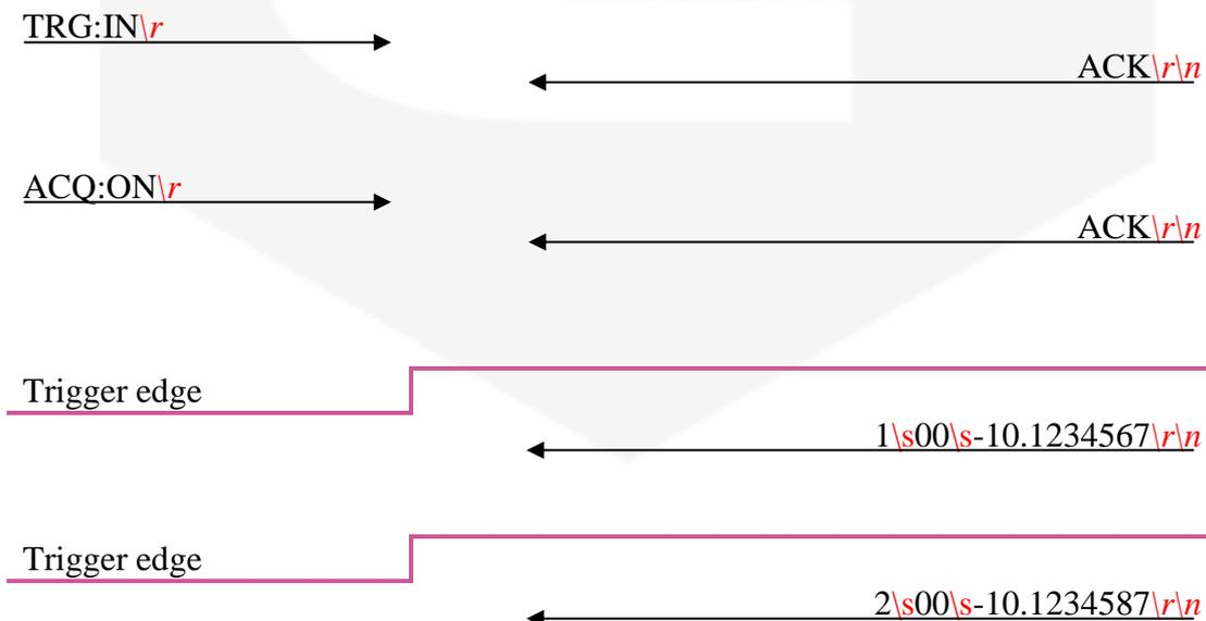
In **Oscilloscope mode** the behavior of the triggered acquisition is different. In this mode the device starts immediately the acquisition after the ACQ:ON command and the rising edge of the trigger input resets the sequence number associated to the
