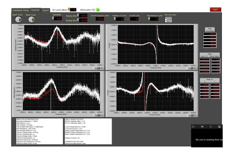
Measured NMR signals with -30dBm at ~40350kHz, and 0.9277Tesla. (the signal can be seen as the small wiggle on phase plot)
