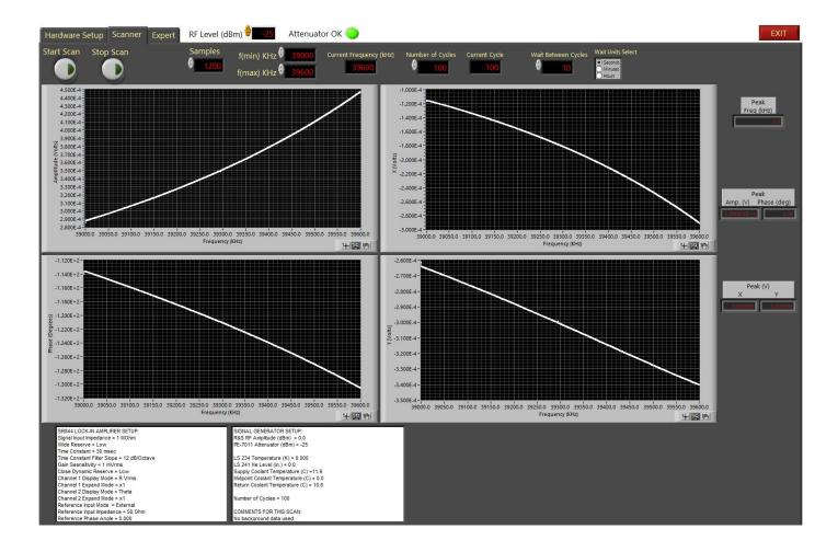
NMR Signal was measured with -25dBm and 0.9277Tesla. The S/N was clearly improved (The potential cost would be more polarization used). The RF jumps, seen more clearly in the previous picture, posed less of the problem now.
