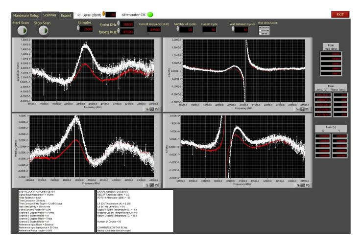
Zoomed in the RF frequency with -30dBm (S~10<sup>-8</sup>V, covered by the noise) and 0.9277Tesla. The averaged signals can be seen, behind live trace, in all 4 plots.
