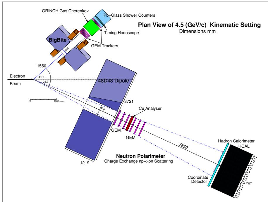
Figure 9: Plan view of experiment  $Q^2 = 4.5 \text{ (GeV/c)}^2$ .
