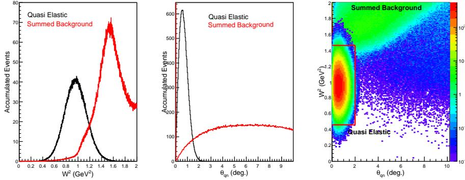
Figure 22: Separation of quasi-elastic and inelastic events for  $d(e, e'n)$  events at  $Q^2 = 4.5$   $(\text{GeV}/c)^2$ . Left: separation in terms of  $W^2$ . Middle: separation in terms of  $\theta_{qn}$ . The QE signal is in black, inelastic background in red. Right:  $W^2$  vs.  $\theta_{qn}$  distributions. Note that the z-scale is logarithmic. The red box shows the area used to select quasi elastic events.
