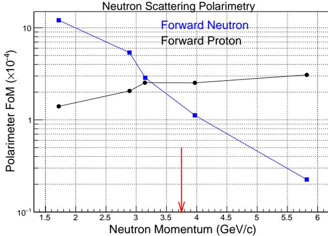
Figure 8: Neutron polarimeter figure of merit as a function of incident neutron momentum for two styles of polarimeter within the SBS apparatus using preliminary data from the recent Dubna measurement. Blue squares: standard  $n - p$  scattering from CH scintillator, black circles: charge-exchange  $n - p$  scattering from Cu. The red arrow marks the neutron momentum at which a charge-exchange measurement of the analyzing power of Cu was made at Dubna.
