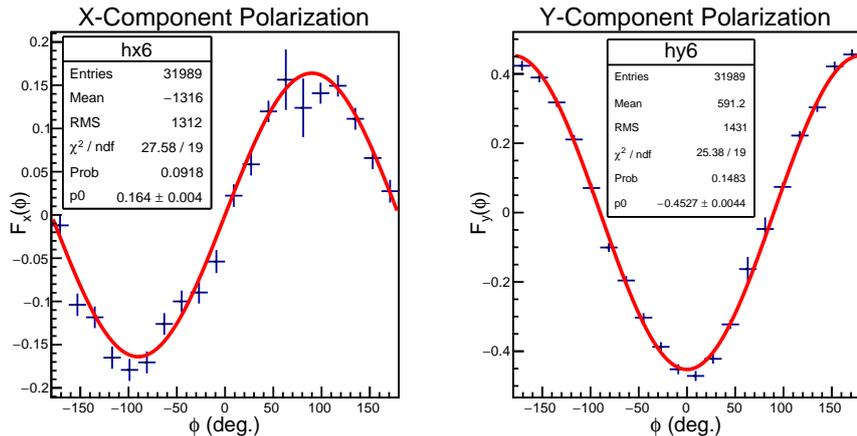
Figure 18: Simulated azimuthal distributions, Eq.15 at an incident neutron momentum of 3.15 GeV/c ( $Q^2 = 4.5$  (GeV/c) $^2$  setting). The red curves are sine and cosine fits to  $F_x(\phi)$  and  $F_y(\phi)$  respectively.
