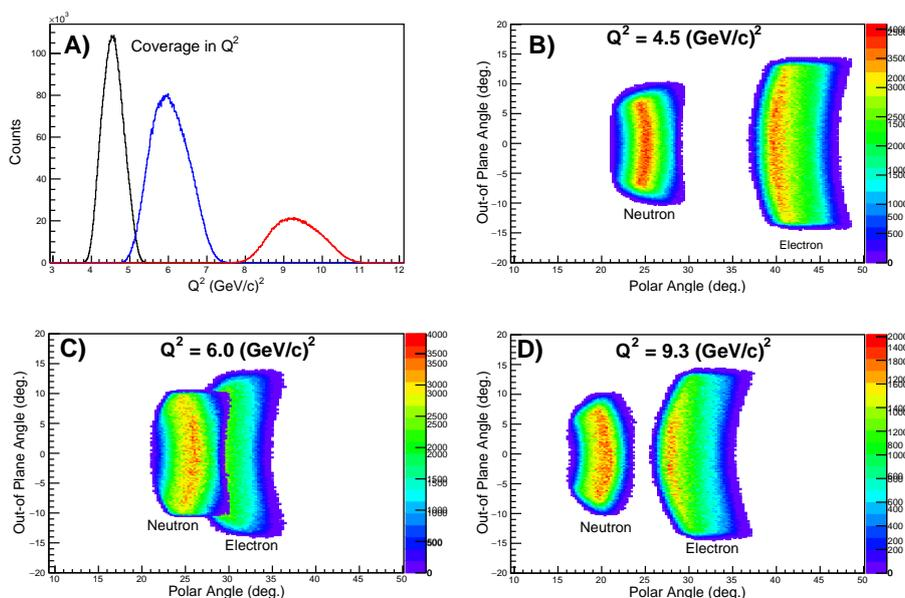
Figure 20: A) range of  $Q^2$  for the nominal settings of Table 3. The distributions are weighted by the Mott cross section. B) electron/neutron angular coverage of BigBite/SBS at  $Q^2 = 4.5$  (GeV/c)<sup>2</sup>. [C) Angular coverage at  $Q^2 = 6.0$  (GeV/c)<sup>2</sup>. D) Angular coverage at  $Q^2 = 9.3$  (GeV/c)<sup>2</sup>].
