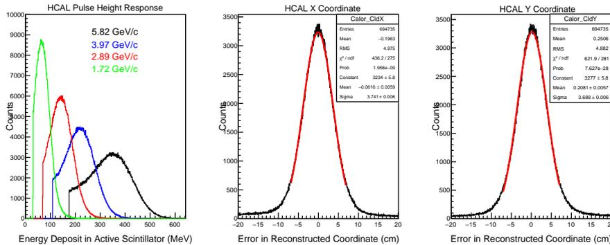
Figure 11: MC calculations of the HCAL response. **Left:** pulse height response for neutron momenta of 1.72, 2.89, 3.97 and 5.82 GeV/c; **middle:** the error in the reconstructed x-coordinate; **right:** the error in the reconstructed y-coordinate.
