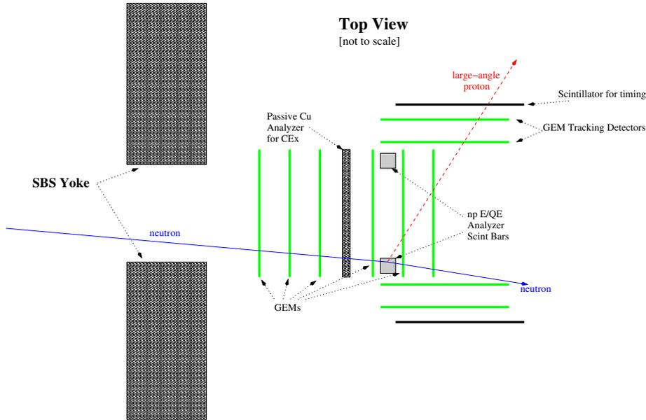
Figure 12: Preliminary schematic of the systems which enable large-angle proton detection within the SBS polarimeter.
