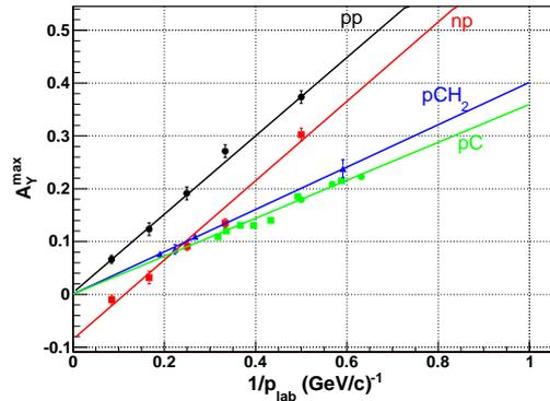
Figure 6: The dependence of the maximum of  $A_Y$  on  $1/p_{lab}$ . Black circles: ANL  $d(\vec{p}, p')n$  data [43, 44]; black line: linear fit. Red squares: ANL  $d(\vec{p}, n)p$  data [43, 44]; red line: linear fit. Blue triangles [46]:  $\vec{p} + \text{CH}_2 \rightarrow \text{charged} + X$ ; blue line: linear fit [46]. Green squares [47] and circles [48]:  $\vec{p} + C \rightarrow \text{charged} + X$ ; green line: linear fit [46].
