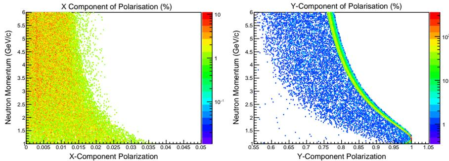
Figure 13: Neutron spin precession as a function of neutron momentum for an initial polarization (0,0,1). Left: induced values of  $P_x$ . Right: induced value of  $P_y$ .
