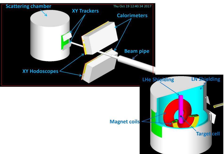
Revised construction of scattering chamber this spring and summer (thanks to J. Zhang)
