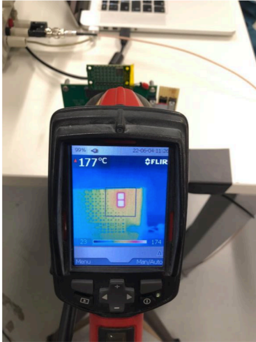
Figure 13: Annealing "in-situ" using reverse bias and Joule effect (left), and comparison of results of the two annealing methods (right).
