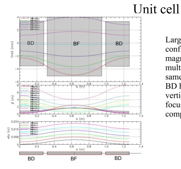
Large momentum acceptance FFA cell, configured with combined function magnets capable of transporting multiple energy beams through the same string of permanent magnets. BD horizontally diverging aka vertically focusing. BF horizontally focusing. Both also have dipole component. Very low dispersion (eta).
