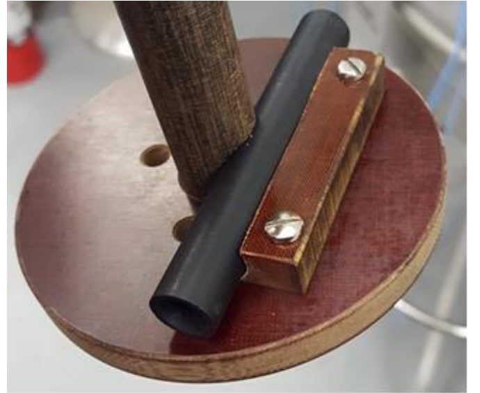
Fig. 3. Bi2223 tube provided by CAN superconductor [10]. The tube and test holder will be inserted inside the bore of a coil providing background field.
