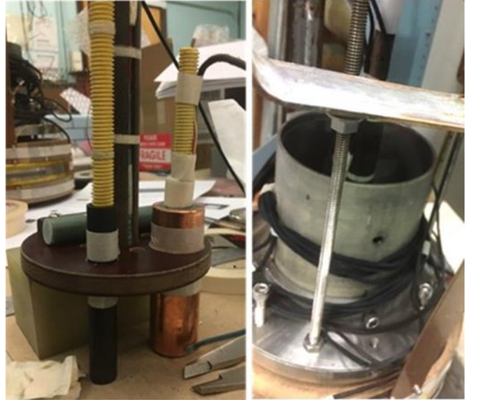
Fig. 8. Left: Disc with tubes of HTS (black) and LTS (copper-clad NbTi), and a center tube holding a Hall probe on the axis of the disc. Right: The disc, with three Hall probes, inside the superconducting coil for testing at 4 K.
