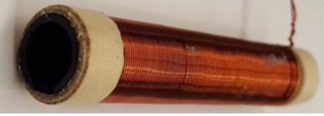
Fig. 5. Copper windings on the HTS tube to immerse it in a field that is primarily axial.
