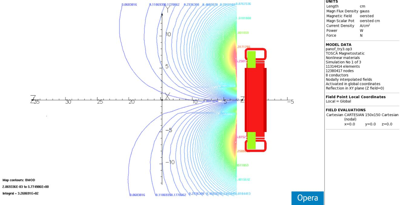
Figure 7. BMODulus in YZ plane at X=0. Discontinuity is still apparent but shape is OK. We'll see what try5 looks like late today.
