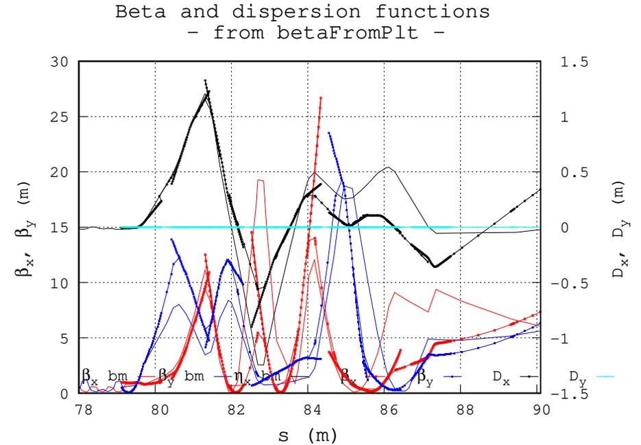
Figure 2: Field maps. Optical functions from field-maps (compared w/ BMAD). Using all 8 quads: I can't get final betas and  $D_x$  tuned concurrently.
