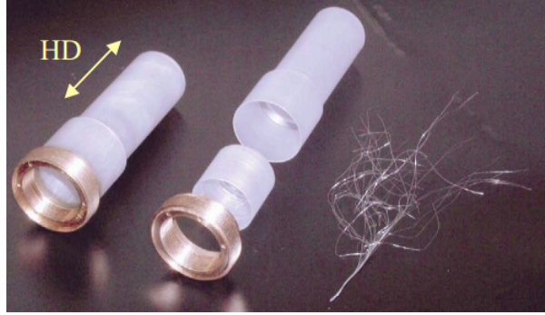
Figure 2.1: Photograph of a deconstructed HDice target, showing the cell, copper ring and aluminium wires [10].
