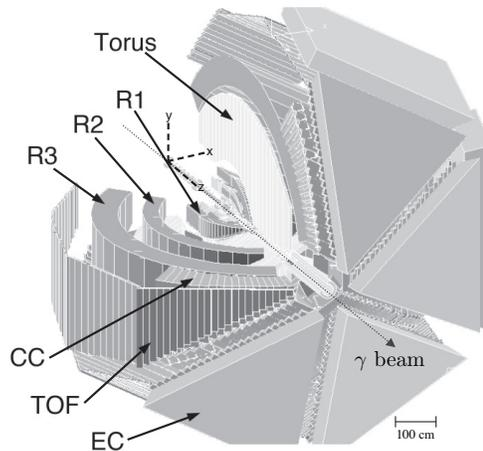
FIG. 1. A perspective view of CLAS showing the torus magnet, the three regions of drift chambers (R1–R3), the Cerenkov counters (CC), the time-of-flight detector (TOF), and the electromagnetic calorimeters (EC). The CLAS reference frame, also indicated here, was defined with the  $z$  axis along the beamline and the  $y$  axis perpendicular to the horizontal. Figure from Ref. [36].
