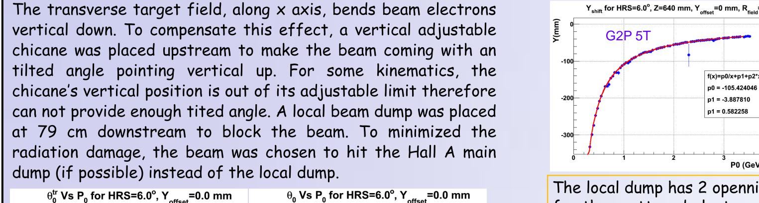
for the scattered electrons to go through, which is also determined by this simulation.
