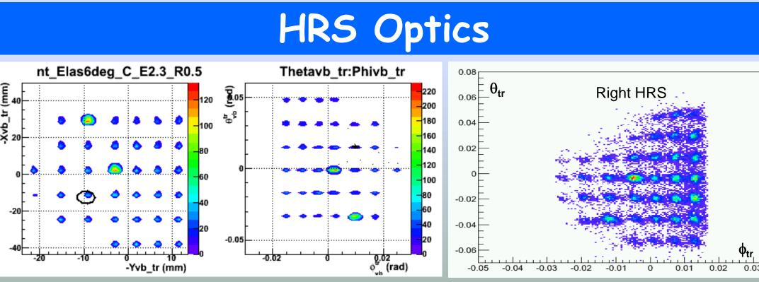
The simulated sieve slit pattern of left HRS (left 2 pannel) and that for the right HRS from the real data (right panel).
