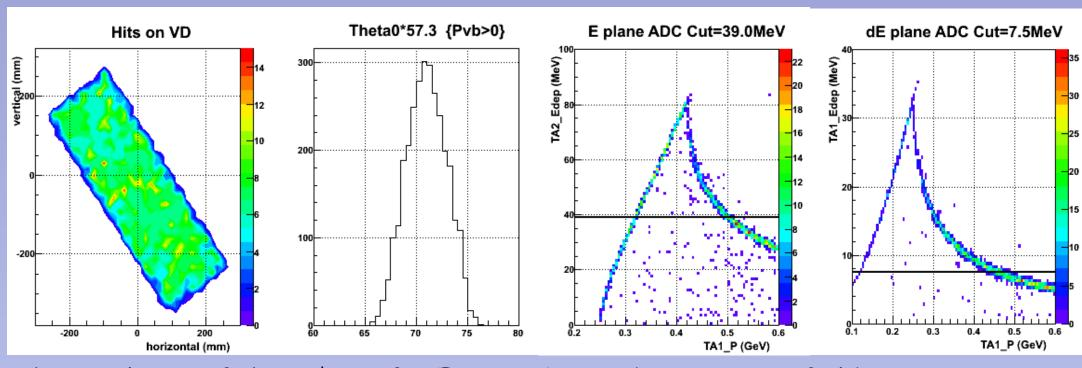
The simulation of the 3<sup>rd</sup> arm for E=2.254GeV and 5.0T target field. Detector was placed at 70 degrees and 210 cm away from the target. Simulated results show that the detector have to be rotated by 16 degrees and the the center of it have to be shift down by 4 cm. The energy thresholds for dE and E plane are 7.5 and 39 MeV, respectivley.
