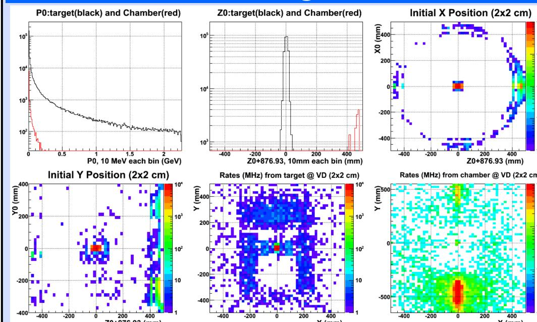
The bremsstrahlung radiation measured at z=90 cm, the back face of the local dump, for E=2.254 GeV and 5.0T target field. The result shows that most of the photon is from the target and a small portion of them are from the target chamber.
