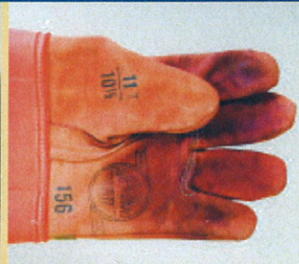
Contamination: Discard protectors contaminated with oil or petroleum compounds.
