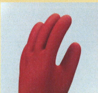
Avoid Storing Inside Out. Storing reversed gloves strains the rubber severely and promotes ozone cutting.
