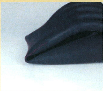
Avoid Folding Electrical Gloves. The strain on rubber at a folded point is equal to stretching the glove to twice its length.
