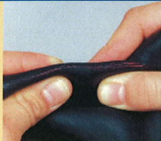
Cracking & Cutting: This type of damage is caused by prolonged folding or compressing.
