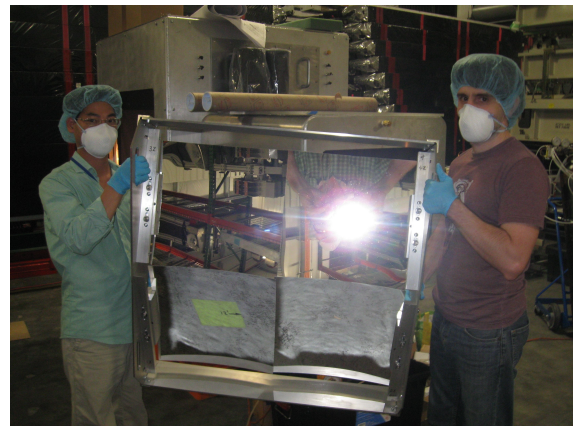
Figure 32: Frame with mirrors about to be moved into tank.
