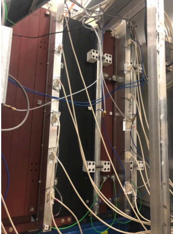
Chambers installed with iron absorbers
