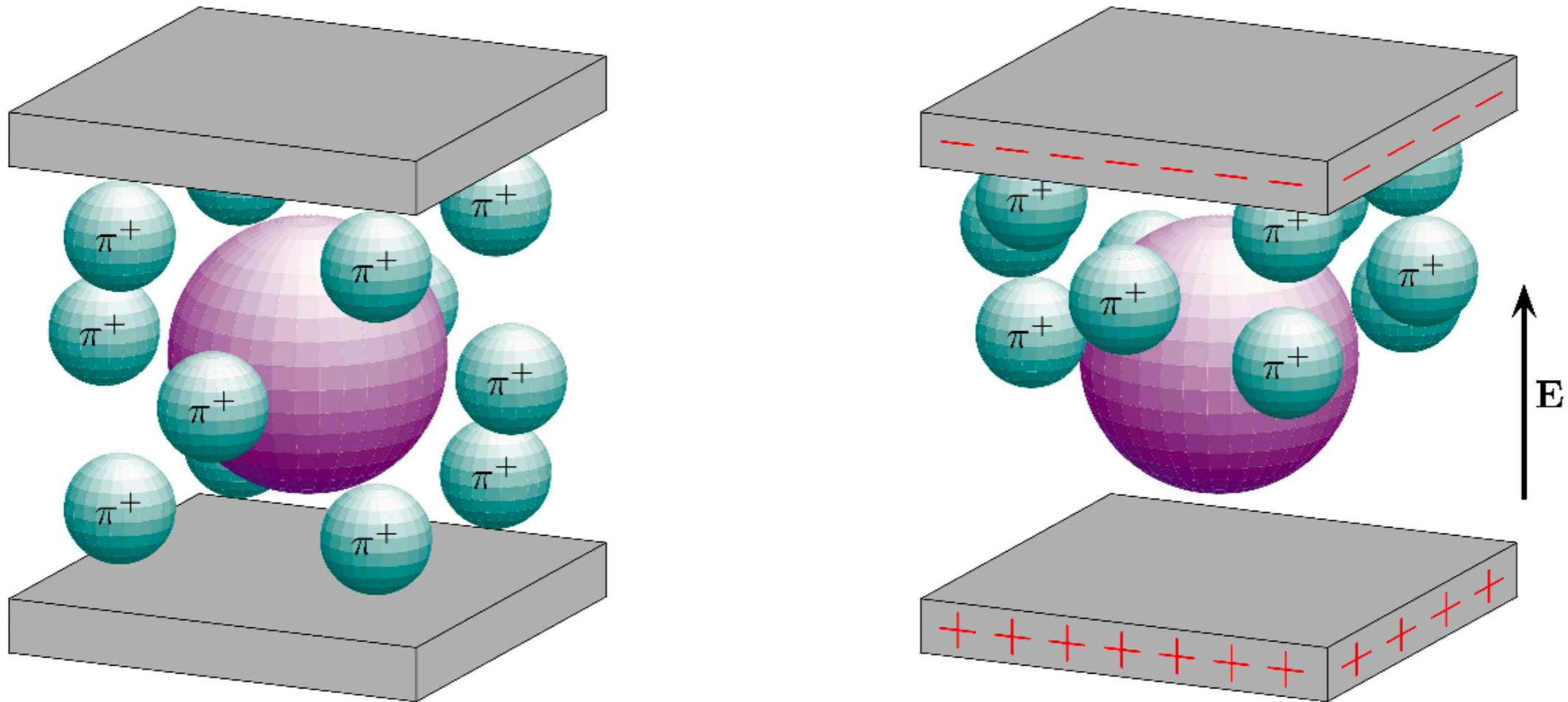
**Electric Polarizability:** proton between charged parallel plates.
