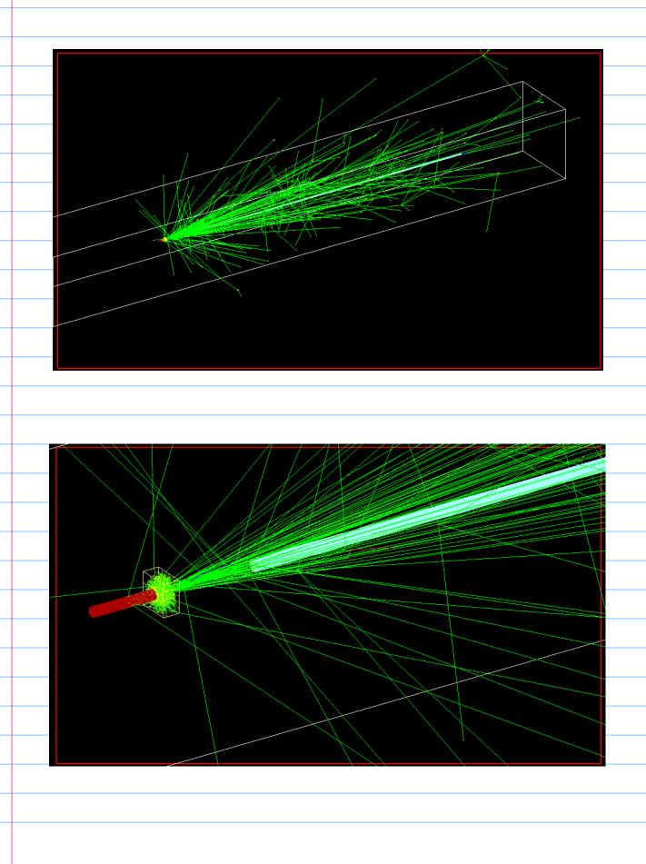
The two plots above represent 1000 thrown Klong with 500MeV/c mometa starting from the center of the Be-procution target.
