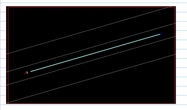
as a first test 10000 Klong are thrown from the center of the Be production target along the z-axis with various momenta and it was registered how often the Klong reaches the liquid hydrogen target. As seen in the list below, at 2 GeV/c momentum the transmission probablity is abut 10% while at 500MeV/c the transmition rate is 7% and at 300MeV/c it is less than 3%.
