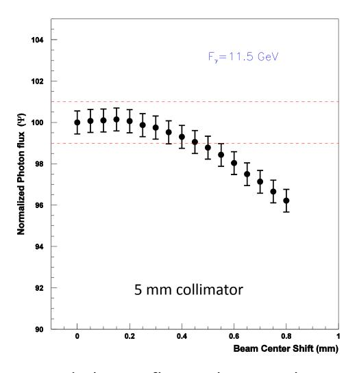
To control the tagged photon flux within 1%, the center of photon beam position should be maintain within  $\pm 200~\mu m$  at primary collimator location
