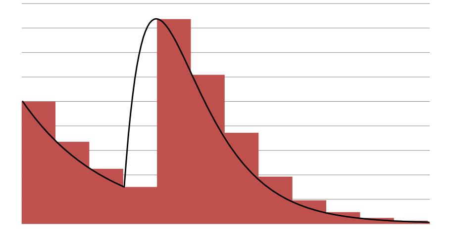
• At a given clock cycle, we consider a "hit" to have occurred if the voltage exceeds some threshold. (Currently  $\approx 5$  MeV). Call this a "threshold event."
