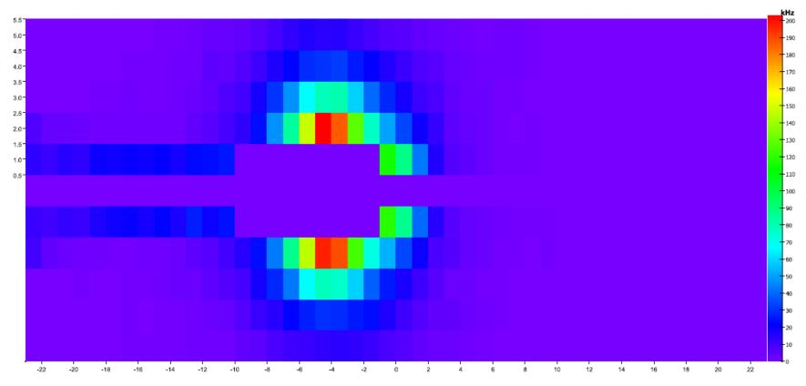
• The "corrected hits" for 6.6 GeV retain some of the electron side "hot spots" still.
