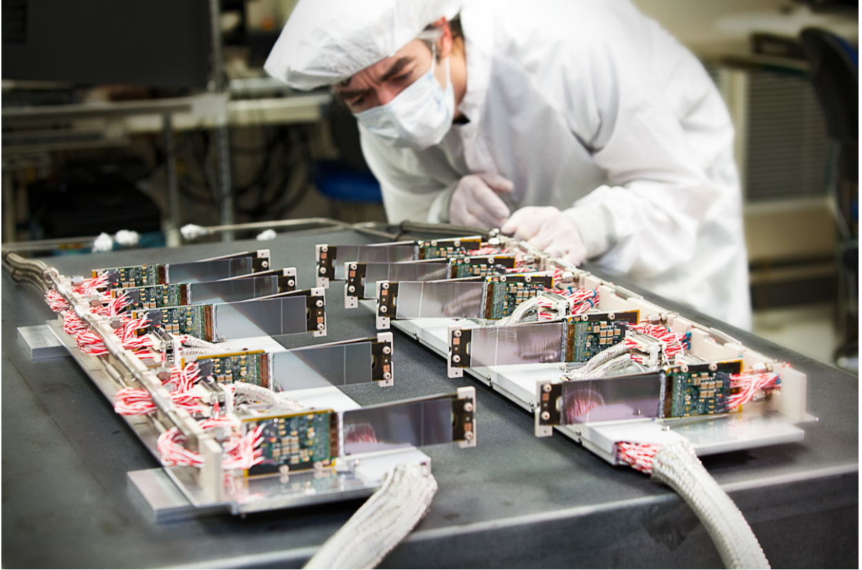
FIG. 13. Both halves of the HPS Test SVT fully assembled at SLAC.
