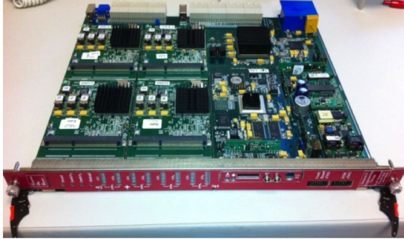
FIG. 23. The Cluster on Board (COB) board, the main board of the SVT DAQ. The RTM is plugged into the COB in the back.
