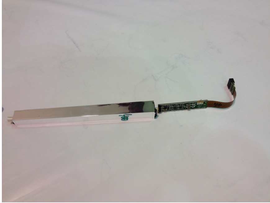
FIG. 18. ECal crystal module consisting of a \text{PbWO}_4 crystal, and APD and a pre-amplifier board.
