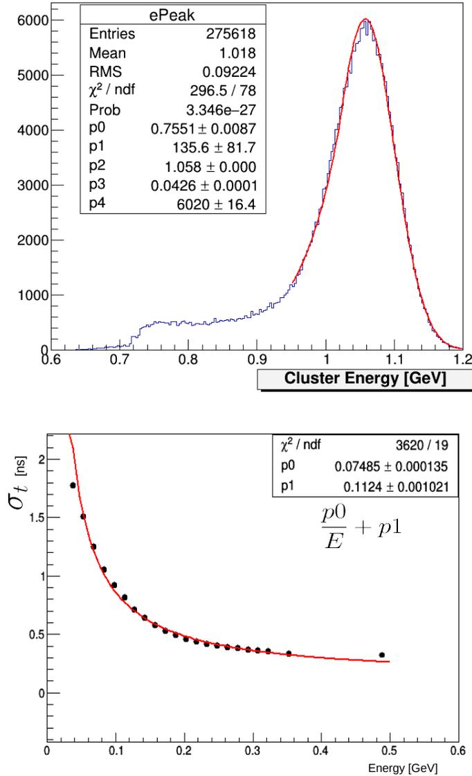
FIG. 2: Reconstructed energy of Coulomb scattered electrons in ECal (top). The energy resolution after the first pass calibration using Coulomb scattered electrons is  $\sim 4.2\%$ . Single channel time resolution as a function of detected energy (bottom).
