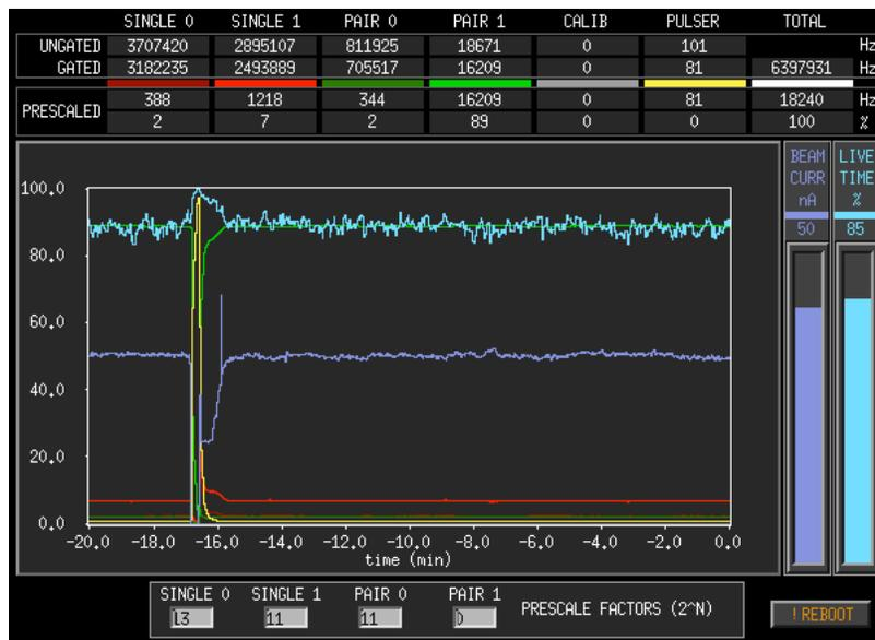
FIG. 3: Online monitoring tool for trigger and DAQ.
