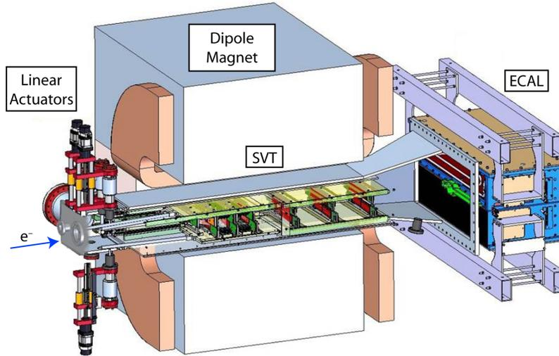
Figure 2: Partial cut-out view of the HPS setup.
