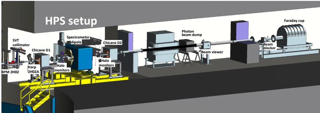
Figure 1: The 2H beam line with the HPS setup.
