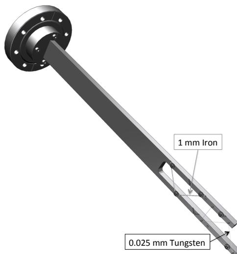
Figure 3: 2H02A Wire Harp. The thin wire is  $25\ \mu\text{m}$  in diameter and the thick wire is 1 mm in diameter. The wire frame is moved into the beam at  $45^\circ$ .
