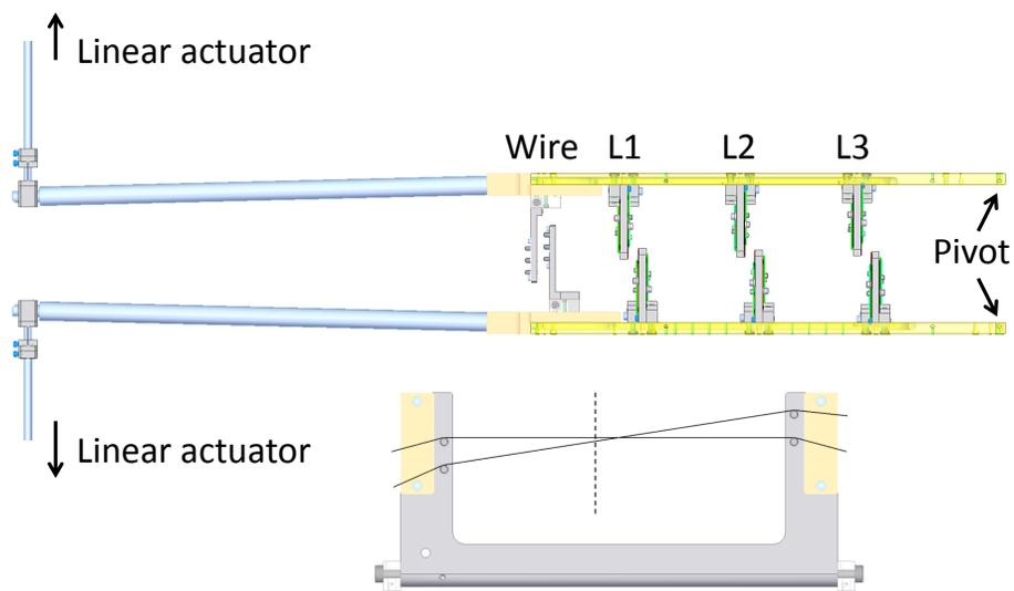
Figure 4: Elevational view of the SVT motion system and beam's eye view of the SVT wire scanner with dashed line indicating the nominal horizontal beam position.
