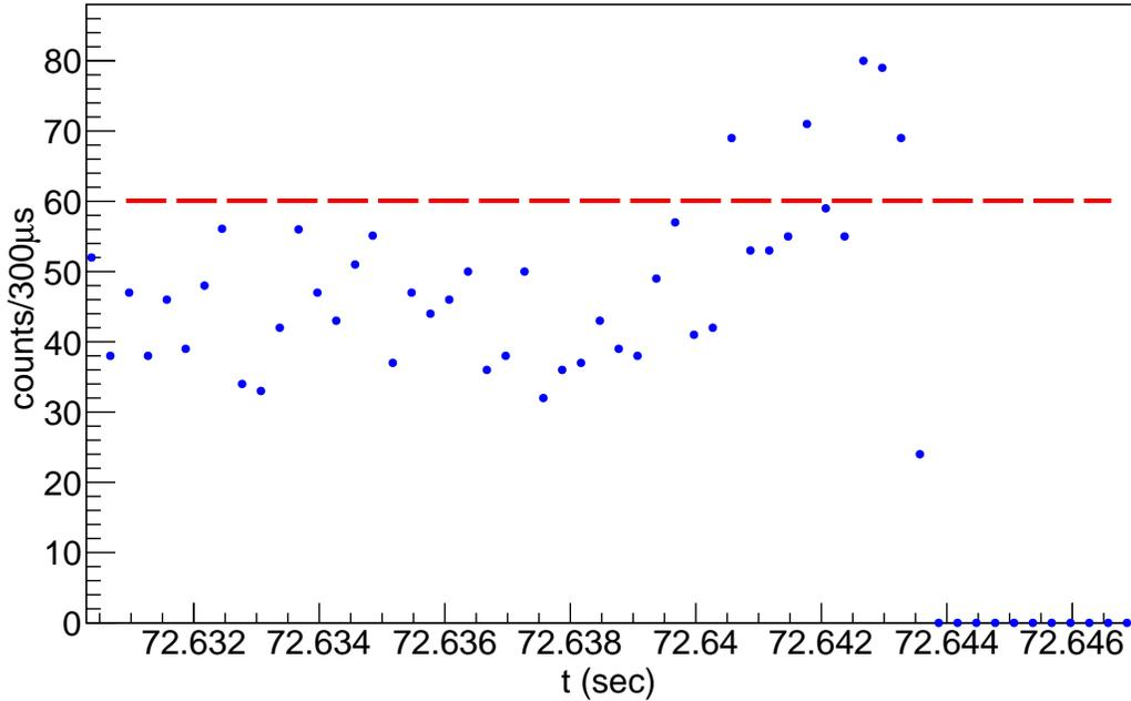
Figure 11: HPS halo counter rates as a function of time. The FSD integration time is 1 *ms* and the beam current is 200 nA. Each point represents integrated counts over a 300  $\mu$ s time interval.
