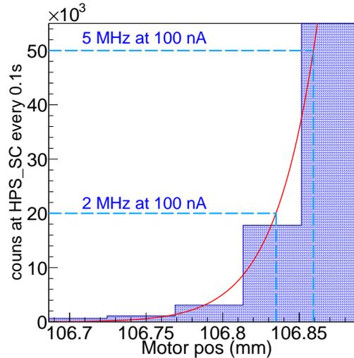
Figure 10: Counts on the halo monitors as a function of harp motor position. The red solid line is the Gaussian fit to the whole beam profile. The two blue dashed vertical lines show position of the wire where rates are 0.2 MHz and 0.5 MHz.
