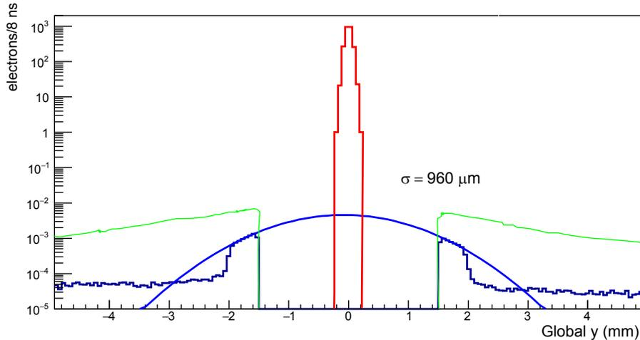
Figure 12: SVT axial layer 1 occupancy during data taking run (green) and no target run (blue). The histogram in red is nominal 50 nA Gaussian core and the blue curve is a Gaussian fit to the halo with  $\sigma$  of 960  $\mu\text{m}$ .
