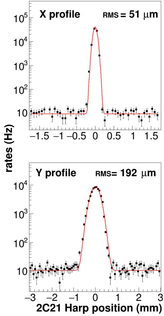
Figure 5: Beam profile measurement with wire harp 2C21.
