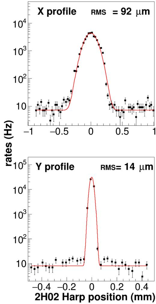
Figure 6: Beam profile measurement with wire harp 2H02A.
