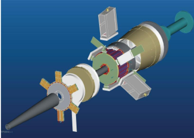
Figure 11: The Forward Tagger (FT) system. The FT provides electron and high energy photon detection in a range of polar angles  $\theta_e = 2.5^\circ - 4.5^\circ$ , and will be fully integrated into the operation of CLAS12.
