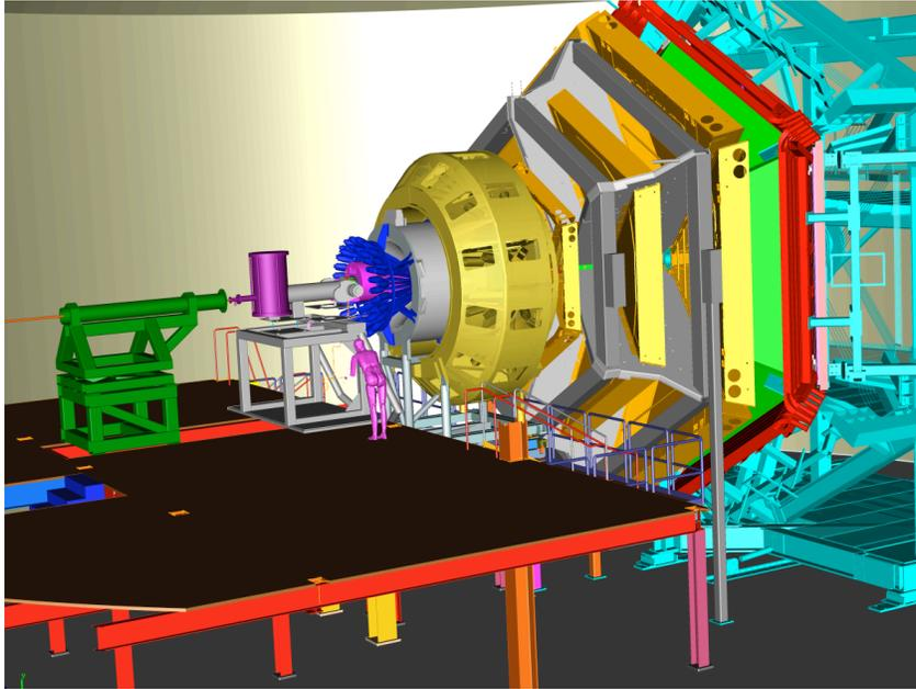
Figure 10: The CLAS12 detector has high hermeticity and high multiplicity reconstruction, can run at high luminosity ( $L > 10^{35} \text{cm}^{-2}\text{s}^{-1}$ ), and is best suited to carry out the proposed experiment.
