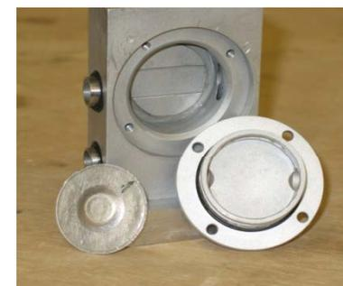
Th-232 target and water cooled high current target holder
