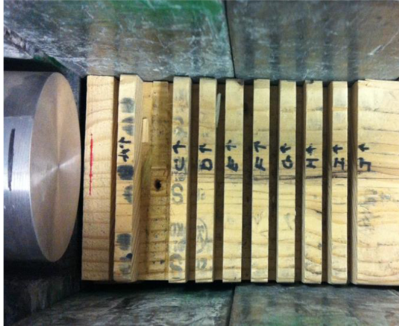
Figure 3.6: Sample positions in front of the HPGe detector.
