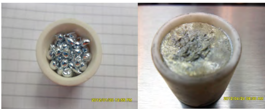
Figure 3.2: 99.99% 40 gram zinc shot in 2\text{ cm} \times 2\text{ cm} alumina cup (left), zinc shot after melting (right).
