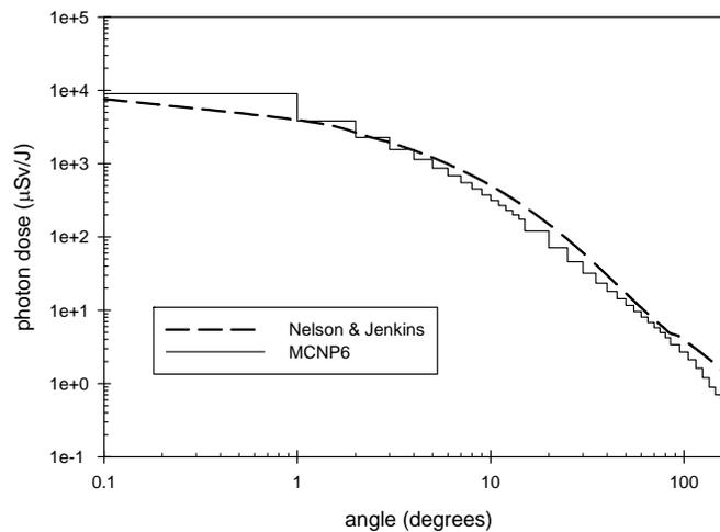
**Figure 5. Photon dose for 7 GeV electrons incident on a 14cm x 10cm copper target.**
