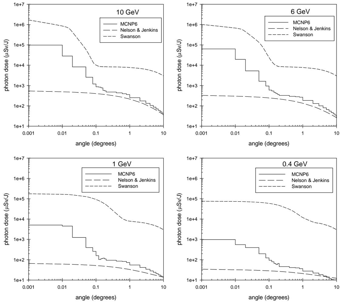
**Figure 4. Photon dose for electrons of selected energies incident on the standard Fe target.**
