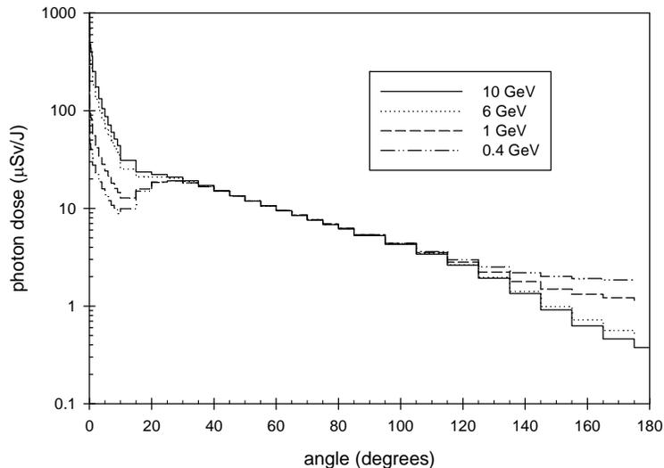
**Figure 3. Photon dose for electrons incident on the standard Fe target calculated with MCNP6.**
