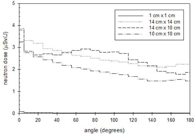
**Figure 6. Neutron dose for selected sizes of a Cu cylinder calculated with MCNP6.**
