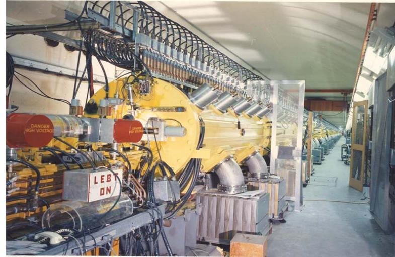
**Figure 3. The BLIP beam line directs protons up to  $115\mu\text{A}$  intensity to targets; generally parasitic operation with nuclear physics programs.**
