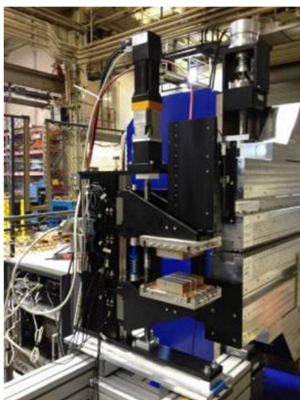
Figure 5. Phase shifter with mounted drive motor
