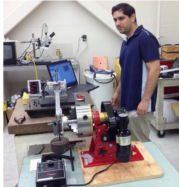
Figure 9. Picture of the undulator pole/flexure fatigue test setup. A motor (foreground) moves a cantilever arm which cyclically loads and unloads the pole flexure. This simulates the load cycles during undulator gap changes.
