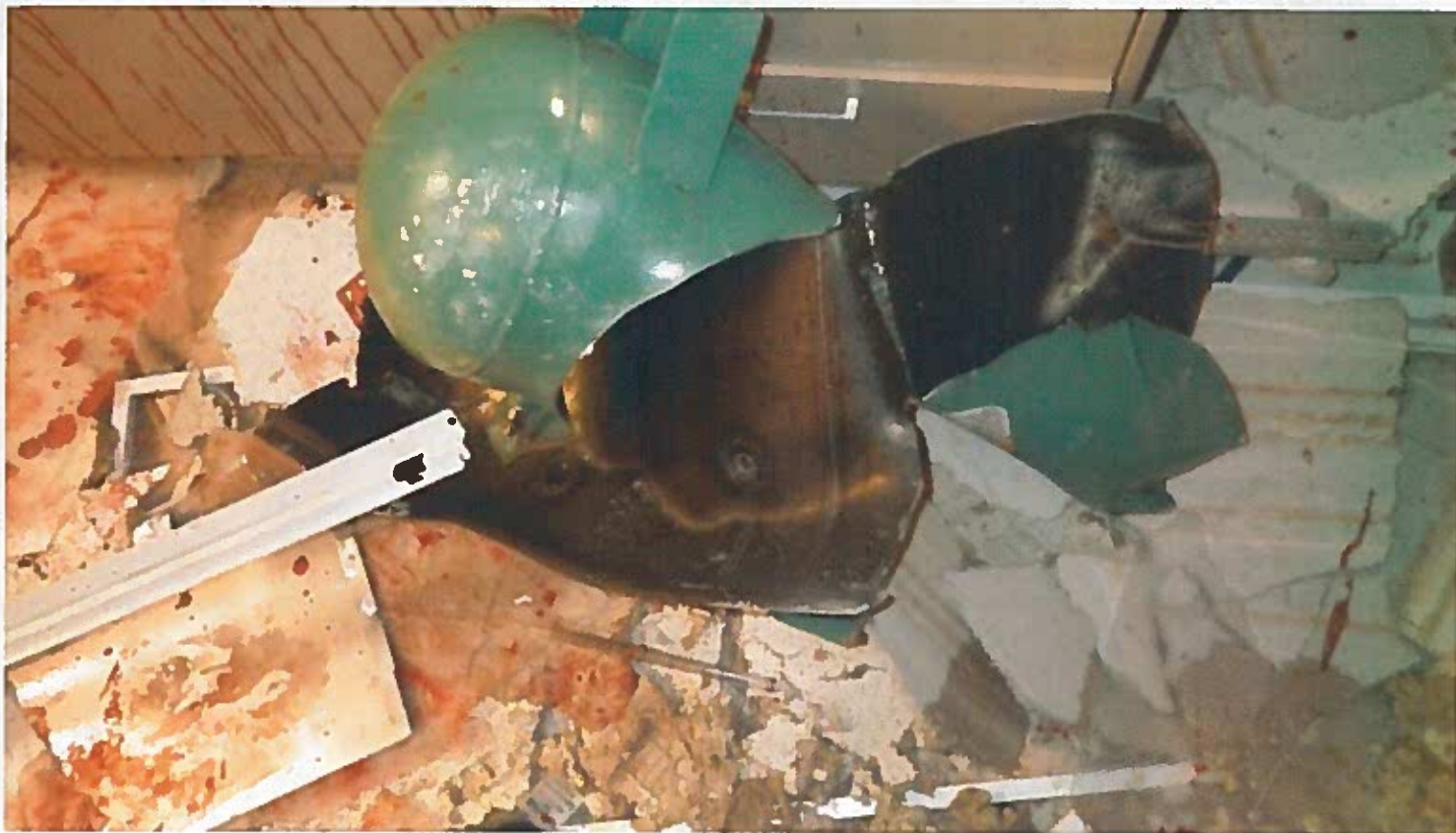
This steel tank ruptured during the explosion, which severed a researcher's arm.
