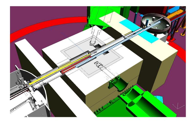
Upstream torus is 2 m long. This "ruler" is 3 upstream torus lengths. It seems to show that the distance from target center to upstream center is only ~ 6m, and the distance from pivot to target center is only approximately 5 m.
